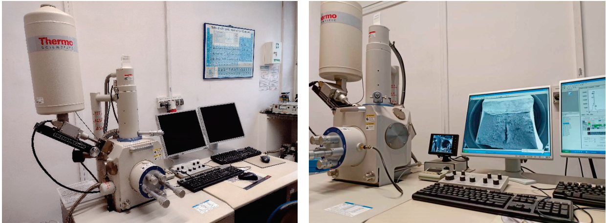
Figure 9. Scanning electron microscope (SEM) used to analyze the microstructure of considered steel.
