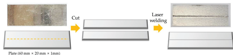
Figure 1. Procedure for laser-welded specimen preparation.
