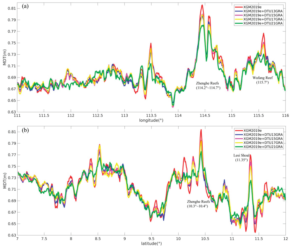
Figure 4. Profiles of various MDTs computed from different gravity field models along latitude 10.4° N (a) and longitude 114.6° E (b). Note: only DTU21GRA was computed with the SAR altimeter data over the study area.
