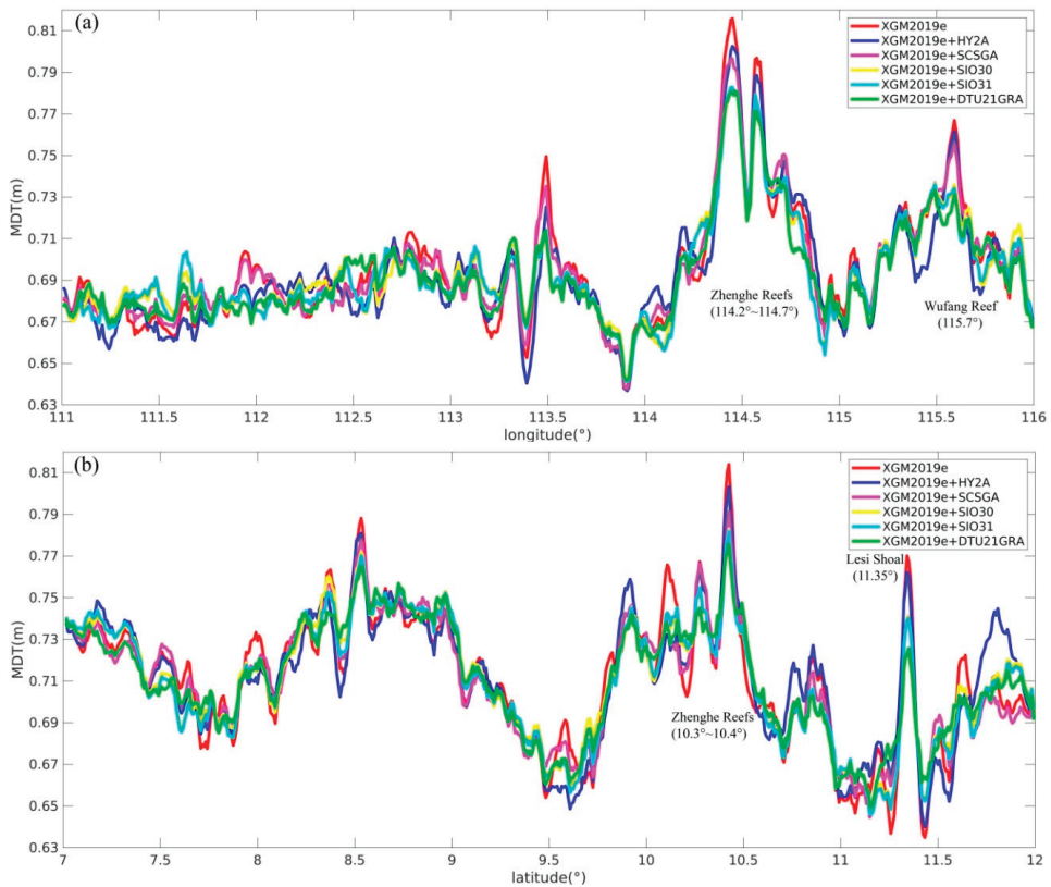
Figure 7. Profiles of various MDTs modeled with different altimetric gravity models along latitude 10.4^{\circ} N (a) and longitude 114.6^{\circ} E (b).
