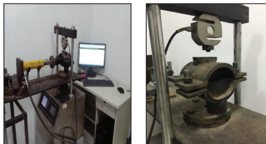
Figure 9. The direct shear test set up.
