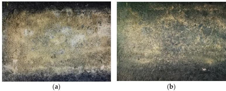
Figure 6. Specimens with a water content of 5% (a) and 10% (b) respectively after adding aeolian sand.
