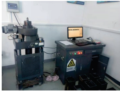
Figure 3. Electro-hydraulic servo pressure testing machine.
