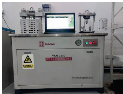
Figure 5. Fully automatic concrete flexural compressive all-in-one.
