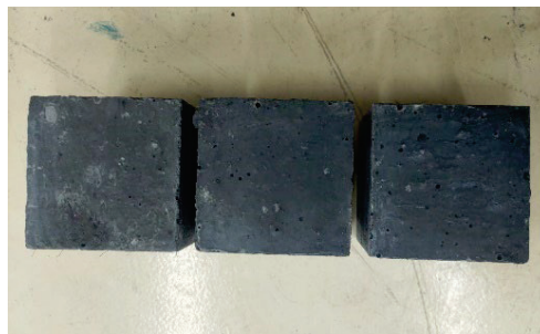
Figure 2. Cubic samples for unconfined compressive strength tests.
