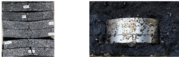
Figure 8. Specimen failure after the three-point bending test.
