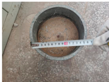
Figure 5. Crushed stone mixture specimen after preparation.
