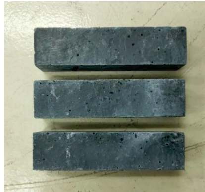
Figure 4. Prism samples for flexural strength tests.
