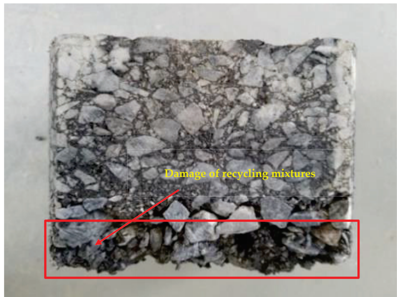
Figure 5. Appearance of cold recycling mixture after loading.
