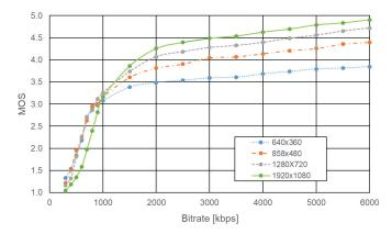
**Figure 6.** Results of the subjective quality assessment (MOS) for the H.264-encoded video as a function of bit rate for different spatial resolutions—measurements in the laboratory.
