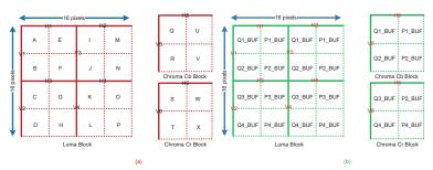
Figure 8. Mapping of pixel blocks to buffers: (a) pixel blocks; (b) buffers.
