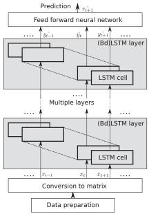
Figure 6. Architecture of the LSTM ANN used for network throughput prediction.
