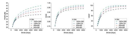
**Figure 14.** Relationship of the objective assessment of video quality encoded in the H.264 standard vs. bit rate for the resolutions  $640 \times 360$ ,  $858 \times 480$ ,  $1280 \times 720$ , and  $1920 \times 1080$ .
