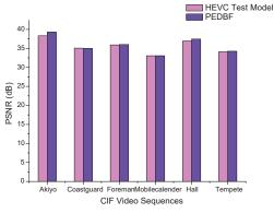
**Figure 18.** Comparison of PSNR with HM for CIF video sequences using QP = 32.
