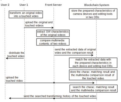
Figure 1. Overall procedure to trace integrity preservation for retouched but non-tampered video file.
