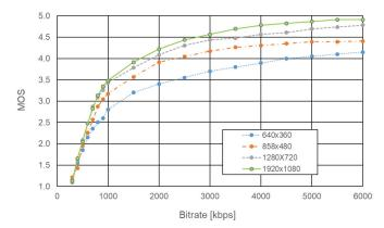
**Figure 9.** Results of the subjective quality assessment (MOS) for the H.265-encoded video as a function of bit rate for different spatial resolutions—measurements in the laboratory.
