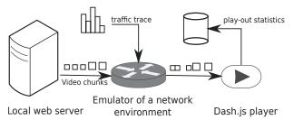
**Figure 10.** Experiment setup includes a web server, the *netem* module and the *dash.js* video player. The connection between the emulated network and the server has fixed parameters. The *netem* module shapes the traffic between the emulated network and the DASH player, providing variable transmission time of video segments.
