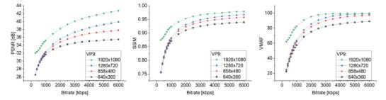
**Figure 16.** Relationship of the objective assessment of video quality encoded in the VP9 standard vs. bit rate for the resolutions  $640 \times 360$ ,  $858 \times 480$ ,  $1280 \times 720$ , and  $1920 \times 1080$ .
