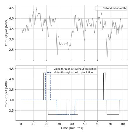
**Figure 12.** Performance of MSS algorithm without and with support of traffic prediction. Throughput prediction eliminates some of the video bit rate drops observed at the beginning, end and approximately the 20th min of the trace. However, as the prediction sometimes overestimates the throughput, the bit rate unnecessarily switches to a higher level at about the 20th min of the trace.
