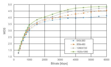
**Figure 12.** Results of the subjective quality assessment (MOS) for the VP9-encoded video as a function of bit rate for different spatial resolutions—measurements in laboratory.
