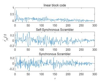
Figure 5. Normalized partial autocorrelation function diagram when SNR = 6 dB.
