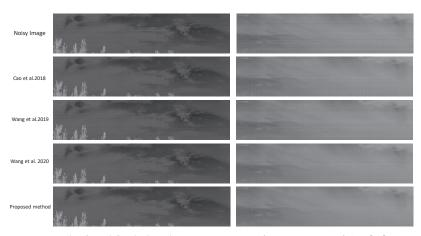
**Figure 9.** Real infrared focal plane linear array non-uniform correction of Cao [16], Wang [17], Wang [18], and our proposed algorithm. The resolution of the presented image is  $1024 \times 4096$  due to the high resolution of the scanned image, as shown in this figure, in order to more accurately compare the denoising effect.
