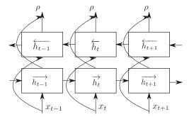
**Figure 5.** Bidirectional architecture of an LSTM network. BdLSTMs apply both forward and backward dependencies.
