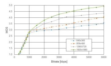
**Figure 5.** Results of the subjective quality assessment (MOS) for the H.264-encoded video as a function of bit rate for different spatial resolutions—measurements at home [49].
