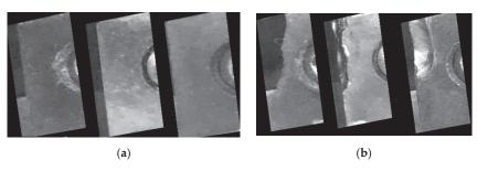
Figure 3. Detected portion of cutting edges: (a) serviceable edges and (b) edges with high wear.
