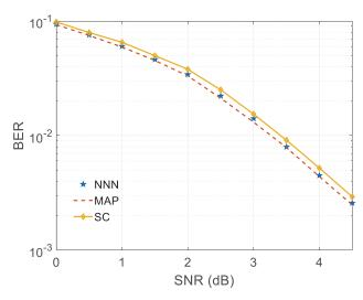
Figure 8. Comparison of the NNN decoding and SC decoding algorithms.
