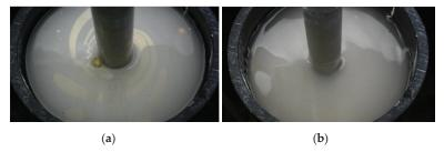
**Figure 2.** Example of surface water in the OS-SS setup showing a (a) "with sheen" image and a (b) "no sheen" image used to create the surface sheen image library for the CNN model development.
