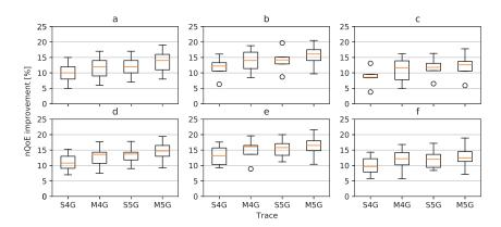
**Figure 13.** The relative improvement of the nQoE metric across different HAS algorithms and network traces with respect to the no-prediction: (a) MSS, LSTM, (b) ExoPlayer, LSTM, (c) Tian, LSTM, (d) MSS, BdLSTM, (e) ExoPlayer, BdLSTM, and (f) Tian, BdLSTM. The nQoE metrics are normalized to the no-prediction case set to 0% improvement. The scenarios with traces from the mobile environment obtain, on average, better results, but their variation is also higher.
