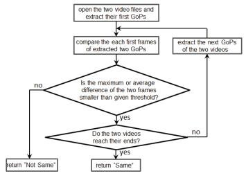
Figure 5. Flow chart of comparison procedure.
