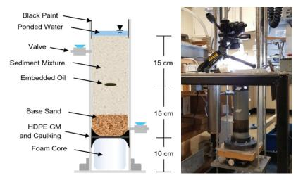
**Figure 1.** Schematic of water-sediment column experimental design including the lighting and image collection in the laboratory OS-SS setup.
