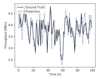
**Figure 8.** One-step prediction for the M5G trace. The prediction tends to overestimate the traffic oscillations, but the unidirectional LSTM ANN achieves better results than a naive predictor based on a simple moving average.
