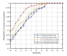
**Figure 15.** Influence of linear block code parameters on the recognition rate under the Condition of Gaussian White Noise.
