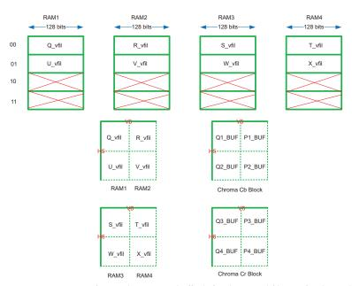
Figure 10. Mapping of internal memory to buffer before horizontal filtering for chroma block.
