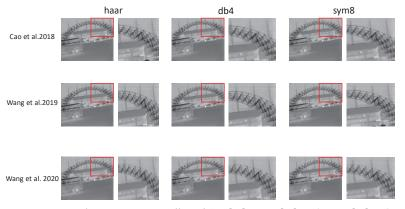
Figure 7. Nonuniformity correction effect of Cao [16], Wang [17], and Wang [18] with respect to distinct wavelet bases. The wavelet bases include "haar", "db4", and "sym8" wavelets. The image "bus" is added with stimulated nonuniformity noise. In order to highlight the correction effect of the algorithm on horizontal stripes and the fuzzy degree of the algorithm on image texture details, the images within the red border are enlarged.
