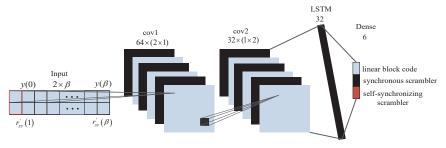
Figure 6. Correlation feature extraction network model diagram.
