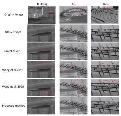
**Figure 8.** Nonuniformity correction effect of Cao [16], Wang [17], Wang [18], and our proposed algorithm. In order to better show the nonuniformity correction effect of each algorithm, this figure selects local magnified images of building, bus, and stairs to compare the effect of each algorithm. The parts in the red circle in the images are the parts where the non-uniform correction results of the contrast algorithm are not good.
