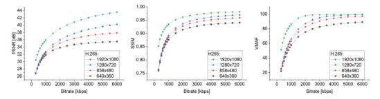
**Figure 15.** Relationship of the objective assessment of video quality encoded in the H.265 standard vs. bit rate for the resolutions  $640 \times 360$ ,  $858 \times 480$ ,  $1280 \times 720$ , and  $1920 \times 1080$ .
