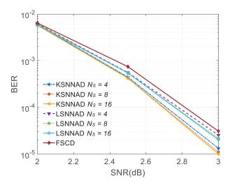
**Figure 13.** Decoding results of different  $N_S$ .
