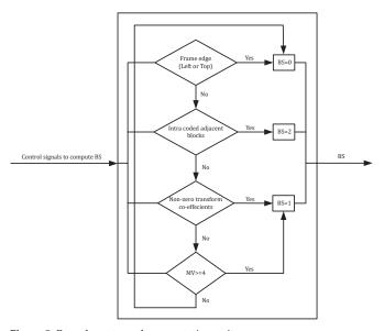
Figure 5. Boundary strength computation unit.
