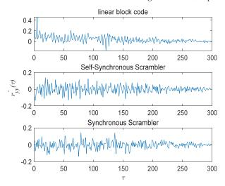
**Figure 4.** Normalized partial autocorrelation function diagram when BER = 0.1.
