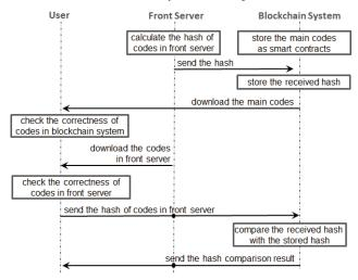
Figure 3. Procedure to check the source code reliability of the proposed scheme.
