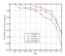
Figure 8. The effect of the number of cells of LSTM on the performance of the algorithm.
