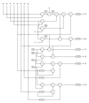
Figure 11. Resource sharing architecture of strong filter—partial view.
