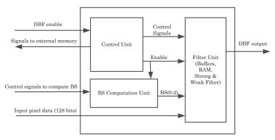
Figure 3. Architecture of V-DPEDBF for HEVC [40].
