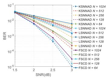
Figure 15. Decoding results of different code lengths.
