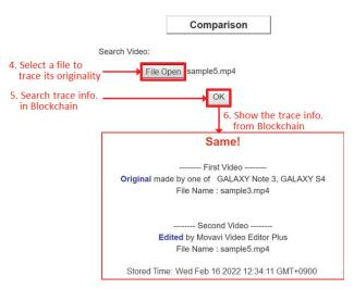
Figure 11. Procedure to search the integrity preservation trace with a hash of input file.
