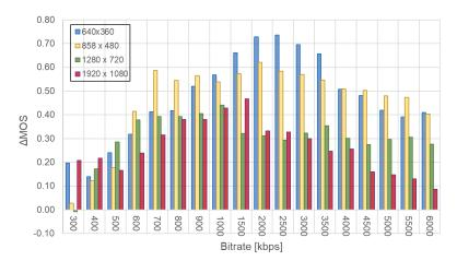
**Figure 13.** Difference between the results of the subjective evaluation of the VP9-encoded video  $(\Delta MOS)$ , conducted in the laboratory and at home, as a function of bit rate for different resolutions.
