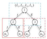
Figure 3. Polar code decoding tree diagram with length 4.
