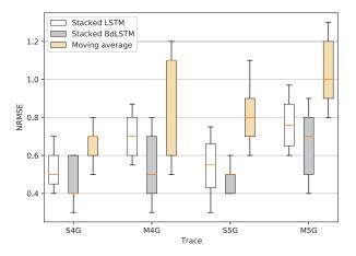
**Figure 7.** NRMSE of the analyzed prediction models for different traces. Every box on the plot represents predictions made on ten overlapping sub-traces every 30 minutes, which were extracted from traces listed in Table 1.
