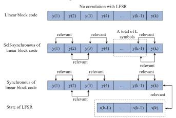
Figure 3. Symbol correlation analysis of linear block code scrambling.
