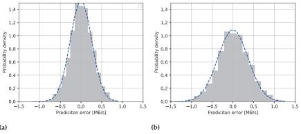
**Figure 9.** Distribution of prediction errors generated by (a) the unidirectional LSTM and (b) a simple moving average for the one-step prediction for M5G trace. The narrower prediction error interval for the LSTM ANN indicates fewer errors and better prediction accuracy.
