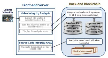
Figure 4. Detailed structure of integrity analysis machanism.
