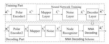
Figure 7. Block diagram of the NNA decoding scheme.
