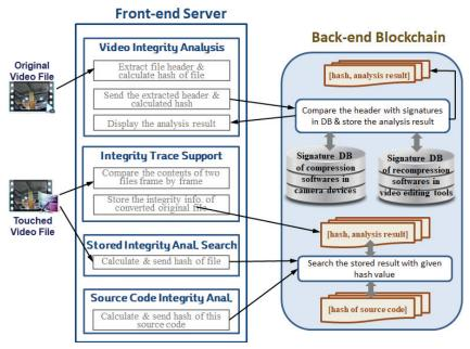
Figure 6. Detailed structure of integrity preservation trace.
