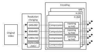
Figure 3. Video sample preparation procedure.
