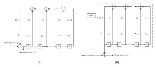
Figure 1. Scrambler schematic. (a) Self-synchronous scrambler; (b) Synchronous scrambler.
