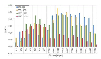
**Figure 10.** Difference between the results of the subjective evaluation of the H.265-encoded video  $(\Delta MOS)$ , conducted in the laboratory and at home, as a function of bit rate for different resolutions.
