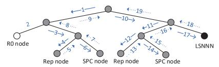
Figure 10. Schematic diagram of the decoding process based on traditional subcodes combined with LSNNN.
