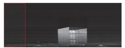
**Figure 4.** Infrared scan image with the addition of Gaussian noise. Due to the very high resolution of the infrared column scan image (3053  $\times$  55,000), only a portion of the scanned image (3053  $\times$  8192) is displayed in this figure. The image within the red border is the image utilized for the linear fitting model in Section 2.1, with a resolution of 3053  $\times$  1500 pixels.
