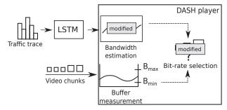
**Figure 11.** The architecture of the *dash.js* reference player. The modified estimation module acquires information about network throughput from the LSTM ANN. The MSS, ExoPlayer and Tian algorithms replaced the player's default playback logic.
