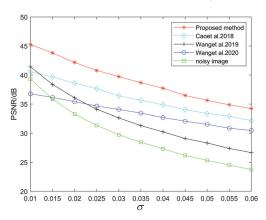
Figure 10. PSNR results of Cao [16], Wang [17], Wang [18], and our method. In order to verify the universality of the nonuniformity correction effect of the algorithm in this paper, 50 images are selected at random from the FLIRADAS dataset, and Gaussian cross-stripe noise with different variance  $\sigma$  is added as shown in Equation (15). The mean PSNR values of the corrected images are calculated using various algorithms to create a relationship curve, as depicted in this figure.
