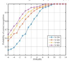
**Figure 16.** Influence of number of samples on the recognition rate under the Condition of Gaussian White Noise.
