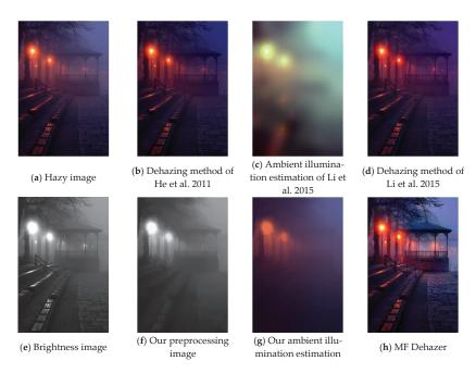
**Figure 2.** Comparison of ambient light estimation and dehazing by different methods. In order to ensure a fair comparison, we use the ambient illumination estimation methods of He et al. [9], Li et al. [26] and MF Dehazer and use the proposed transmission estimation method to remove haze to compare the effects of different ambient illumination estimation methods.
