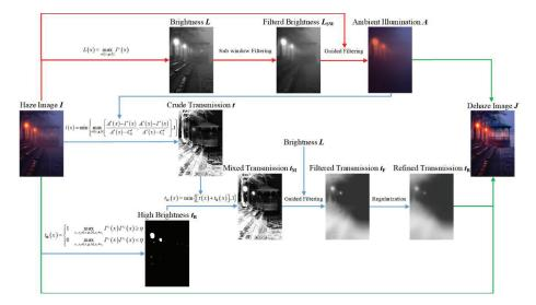
**Figure 1.** Flow chart of the proposed dehazing method. In this chart, the red line is the ambient illumination estimation method, the blue line is the transmission estimation method, and the green line is the result.
