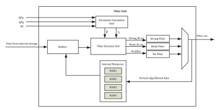
Figure 6. Filter unit of dual-edge deblocking filter architecture.
