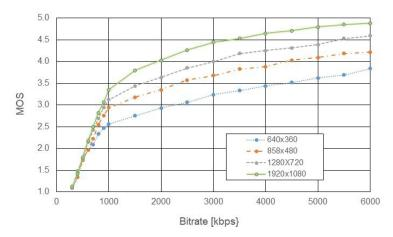
**Figure 8.** Results of the subjective quality assessment (MOS) for the H.265-encoded video as a function of bit rate for different spatial resolutions—measurements at home.
