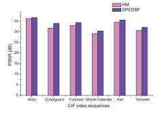
**Figure 22.** Comparison of PSNR with HM for CIF video sequences using QP = 37.
