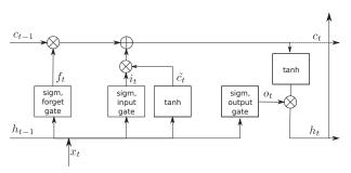
**Figure 3.** Structure of LSTM memory block:  $x_t$  is an input signal at the time t,  $c_{t-1}$  and  $c_t$  represent cell states at the previous t-1 and actual t times,  $h_{t-1}$  and  $h_t$  are output signals of the cell at t-1 and t times, t represents the bias. The symbol t represents the multiplication and t summation of signals.
