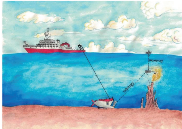
Figure 2. Sketch of the MEED in operation.
