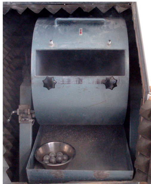
Figure 8. Los Angeles testing machine with steel balls in the front (in soundproof enclosure).
