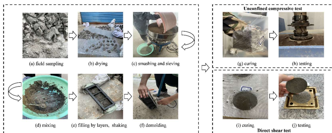
Figure 7. Specimen preparation procedures of unconfined compressive and direct shear tests of cemented soil.
