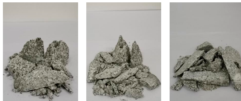
Figure 31. Fracture morphology of disturbed samples after impact failure.
