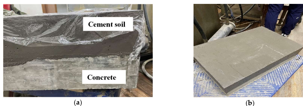
Figure 4. Cemented soil–concrete interface sample. (a) Interface sample before curing, after preparation; (b) Interface sample before testing, after curing.
