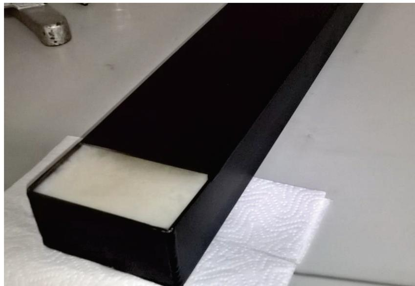
**Figure 7.** Thermal energy battery containing a new PCM in the form of a eutectic mixture.
