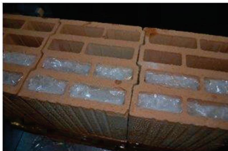
**Figure 5.** Example of using PCM packages in ceramic hollow bricks [55].
