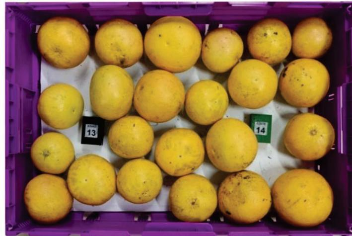
**Figure 4.** Crate outfitted with PCM alveoli, loaded with oranges, and equipped with sensors for data acquisition.
