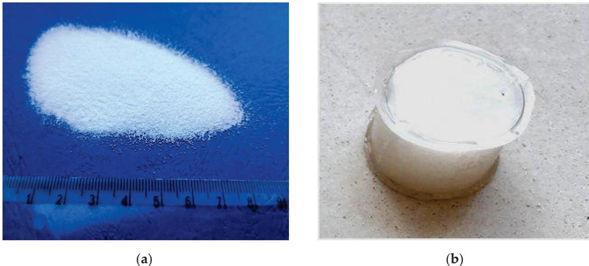
**Figure 3.** (a) Image of Micronal—a coated PCM microgranulate; (b) stable capsule with an organic phase change material.
