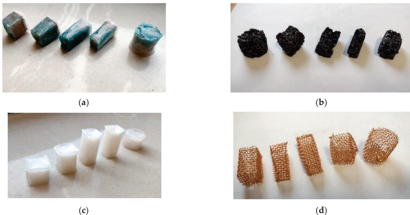
**Figure 8.** (a) Compact thermal energy batteries with a PCM and copper conductor; (b) conductor coke recycle; (c) compact thermal energy batteries with a pure PCM; (d) thermal energy battery conductor framework made of copper mesh.
