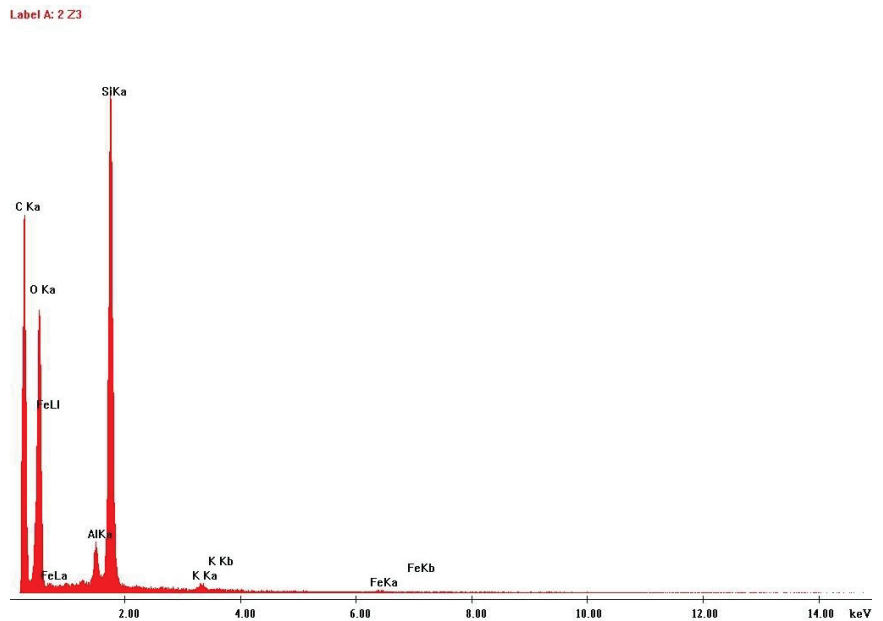
Figure 10. EDS analysis results: Airborne sample collected on polycarbonate filter.
