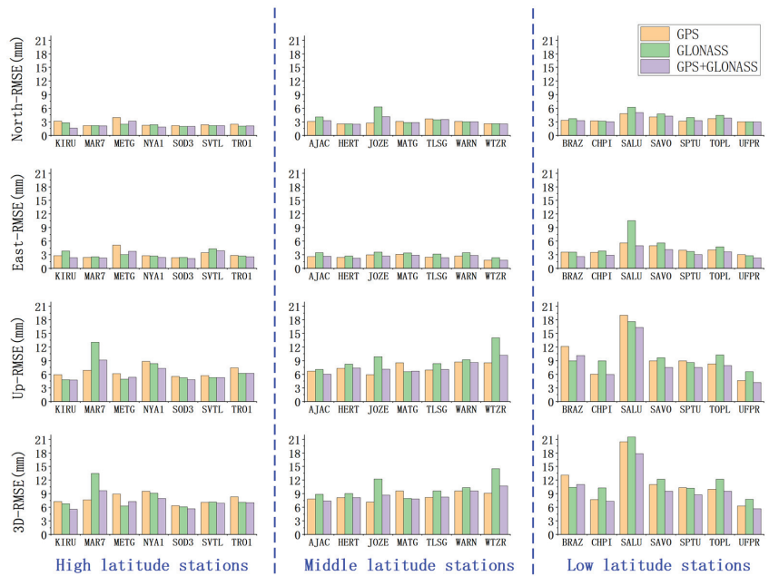
Figure 13. The RMSE of coordinates of all the stations estimated with PPP.
