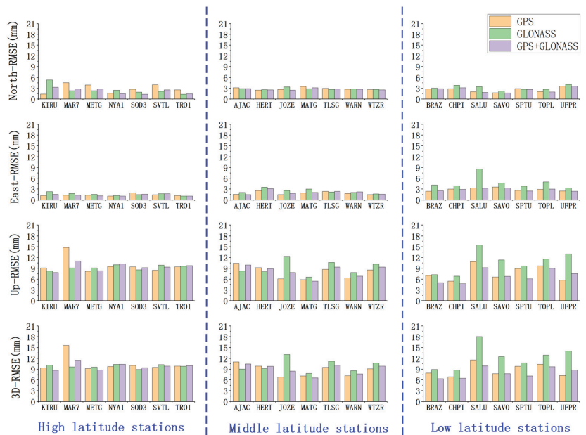
Figure 9. The RMSE of coordinates estimated with DD processing.
