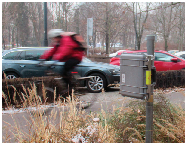
Figure 1. Microwave radar installed next to a bicycle lane (own study).
