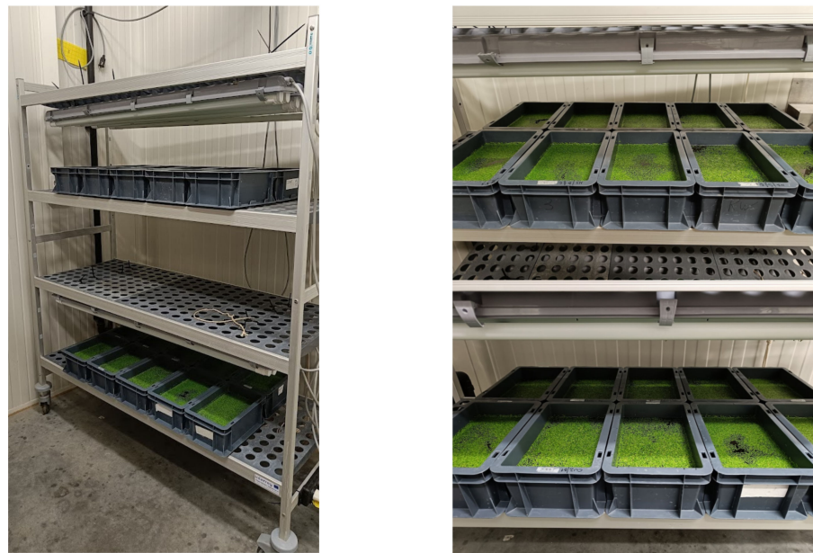
Figure 7. Picture of the growth rack used for all tray experiments, with 10 PET containers and 4 parallel TL-lights per level.
