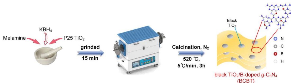
Scheme 1. Schematic illustration for synthesis of the black TiO 2 /B-doped g\text{-C}_3\text{N}_4 (BCBT).
