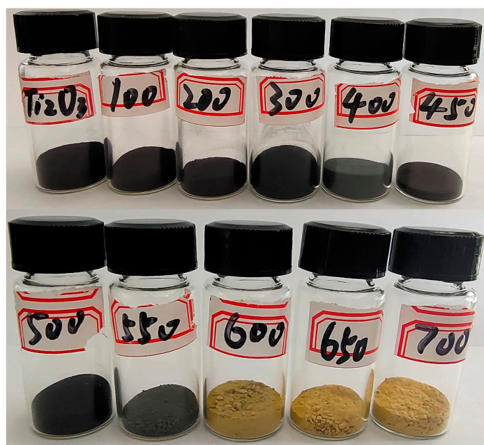
Figure 2. Optical photos of \text{Ti}_2\text{O}_3 at different heat treatment temperatures.
