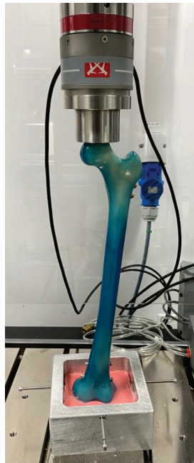
Figure 2. Experimental setup for measuring the stiffness and failure load after creating the osteoporotic femur models with different proximal interlocking screw constructs.
