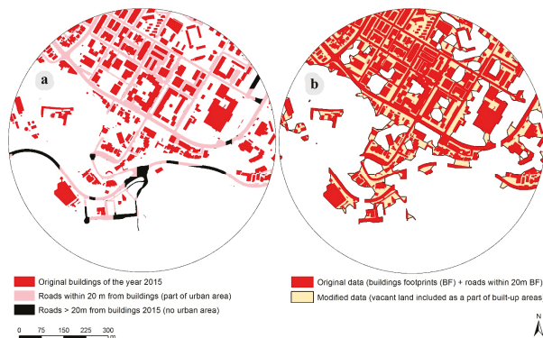
Figure 3. Delineation of built-up areas: (a) selected roads as a part of urban areas in pink, roads within 20 m of building footprints; rejected roads as a part of urban areas in black, roads more than 20 m from building footprints; (b) outputs of urban areas delineation (both the yellow and the red areas are considered as built-up areas).
