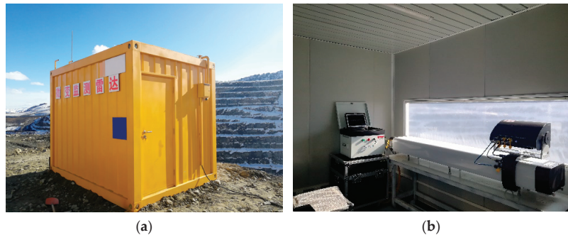
Figure 2. (a) micro-deformation monitoring radar protection device; (b) micro-deformation monitoring radar.
