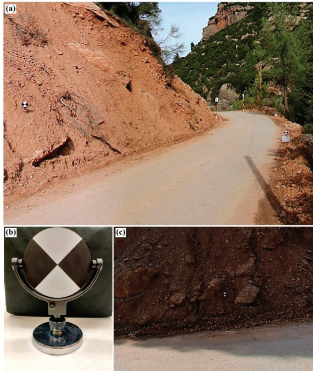
Figure 5. (a) Distribution of GCPs in the area of interest, (b) 4.5" black and white target, (c) 4.5" black and white target within the landslide area.
