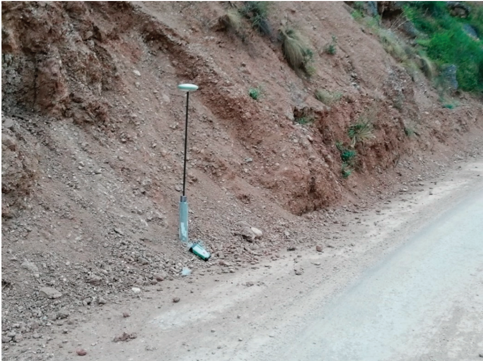
Figure 4. Permanent location on the road area for the execution of GNSS measurements.
