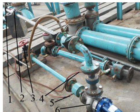
Figure 3. Experimental device: (1) valve in the outlet, (2) flowmeter, (3) valve in the inlet, (4) pressure transducer in the outlet, (5) pressure transducer in the inlet, (6) pump.
