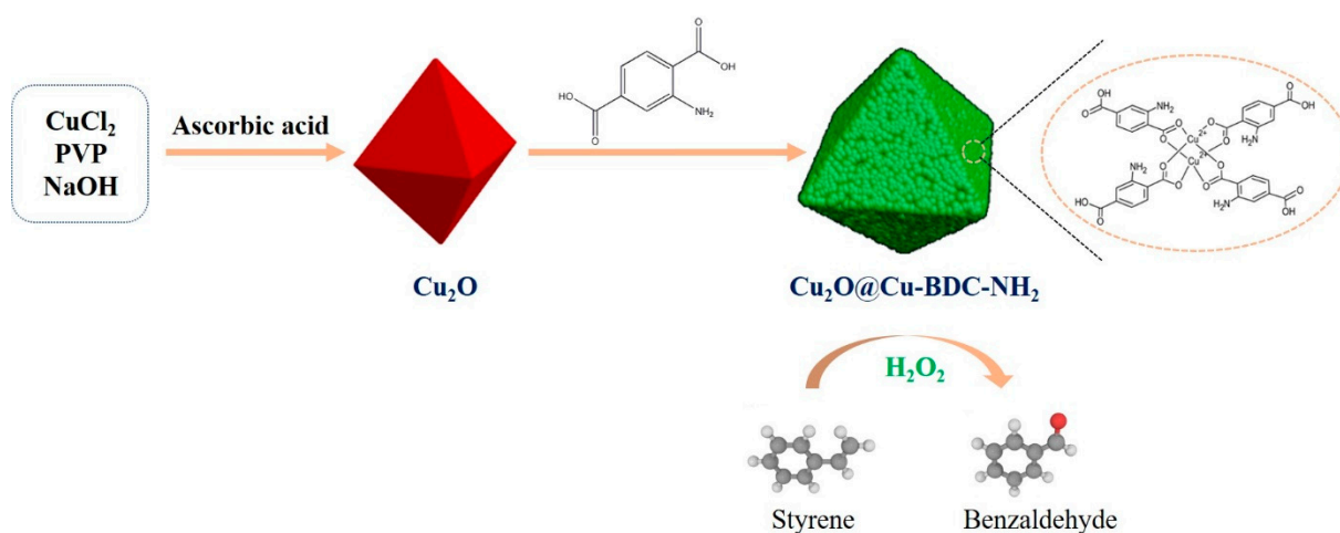
Scheme 1. The illustration of the synthetic process from Cu 2 O toward Cu 2 O@Cu-BDC-NH 2 for the selective oxidation of styrene with H 2 O 2 as green oxidants.
