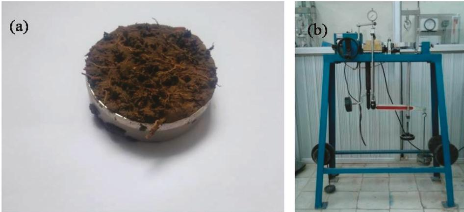
**Figure 5.** Experimental setup for determining the direct shear strength of the soil: (a) soil sample; and (b) experimental device for measuring the direct shear strength (photos were taken on 26 May 2016).
