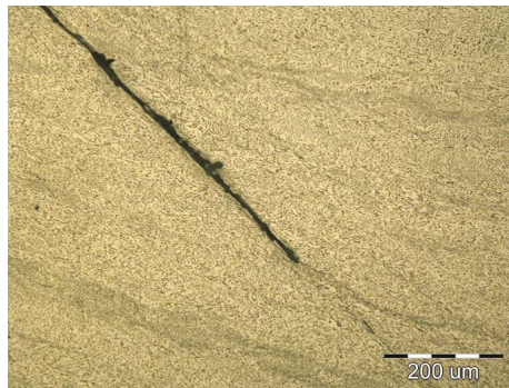
Figure 9. Microstructure of specimen deformed at 700 °C/1 s -1 of the as-rolled Ti-55 alloy.
