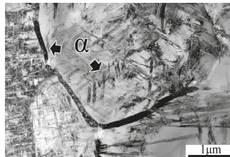
Figure 2. Transmission electron microscope (TEM) image of the alloy after thermomechanical processing.
