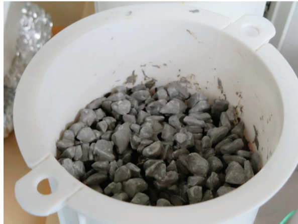
Figure 7. Experimental porous concrete column measuring 10 cm in diameter and 10 cm in depth.
