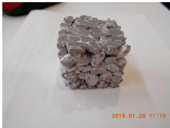
Figure 8. Porous concrete cube with each side measuring 4 cm.
