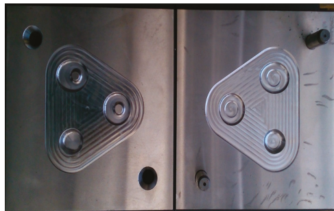
Figure 16. Manufactured forging dies.
