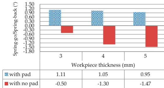
Figure 7. Comparison of the predicted spring-back/spring-go between the cases of U-bending with and without pressure pads, with respect to workpiece thicknesses ( \theta : 90^\circ , R_p : 5 mm, W : 30 mm, WP_L : 120 mm, R_{ud} : 5 mm).
