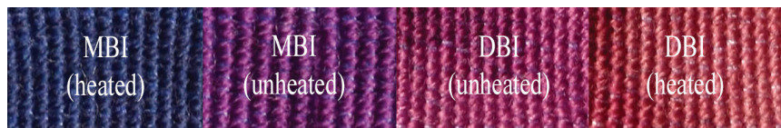
Figure 1. (Left to right) MBI-dyed wool heated in water, MBI-dyed wool with no heat application, DBI-dyed wool with no heat application, DBI-dyed wool heated in water [7].
