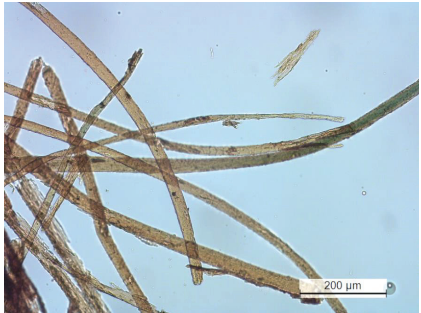
Figure 3. Wool fibers of the shawl's warp band with some visible scales and blue dye.
