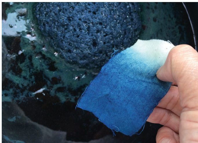
Figure 15. The third day, later. Testing of the coloring power of the vat with a sample of cotton cloth (photo H. Sumi).
