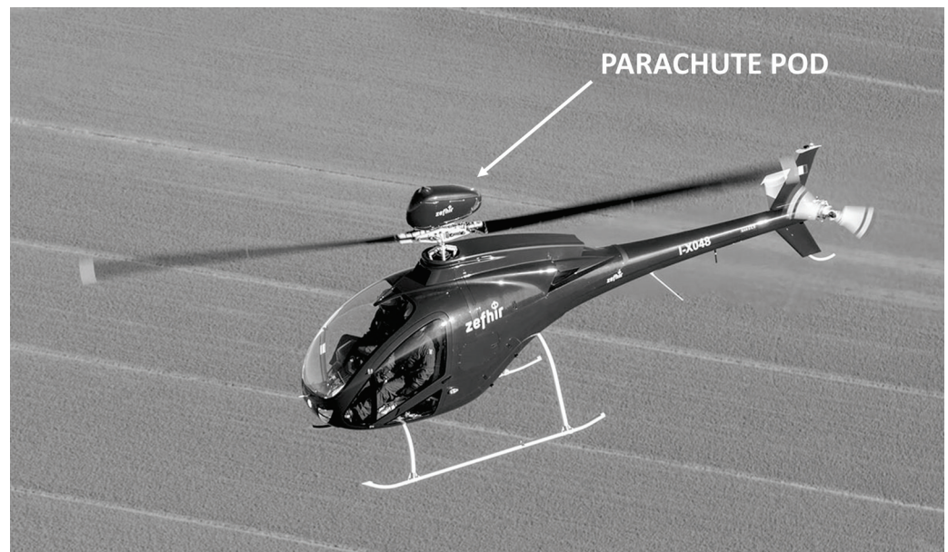
Figure 1. Zephyr helicopter (courtesy of Curti Aerospace Division).
