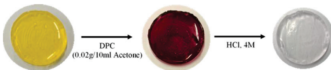
Figure 11. Regeneration method of silica-based xerogel.
