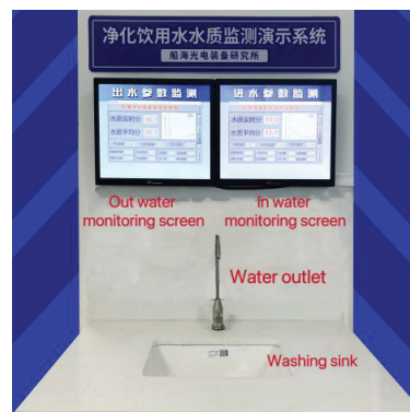
Figure 4. The drinking water quality monitoring demonstration system.
