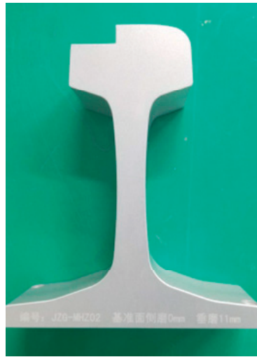
Figure 14. Standard worn rail with a vertical wear of 11.00 mm. (NO. JZG-MHZ02, horizontal wear 0 mm, vertical wear 11 mm).
