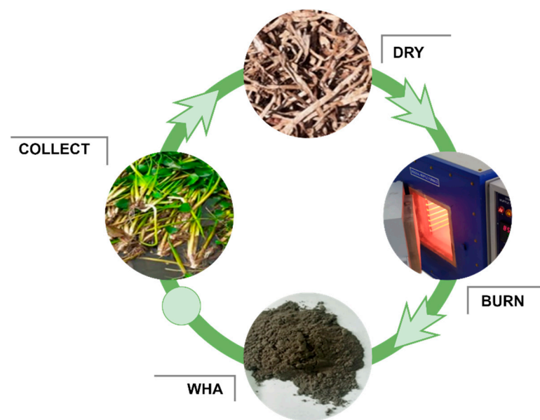
Figure 2. Main steps of the WHA production process.
