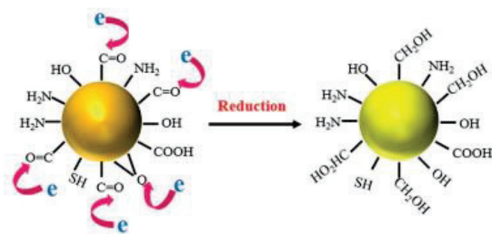
Figure 20. Conversion of CDs to r-CDs by C=O reduction to CH 2 OH groups (adapted with permission from [62], copyright 2015 Royal Society of Chemistry).
