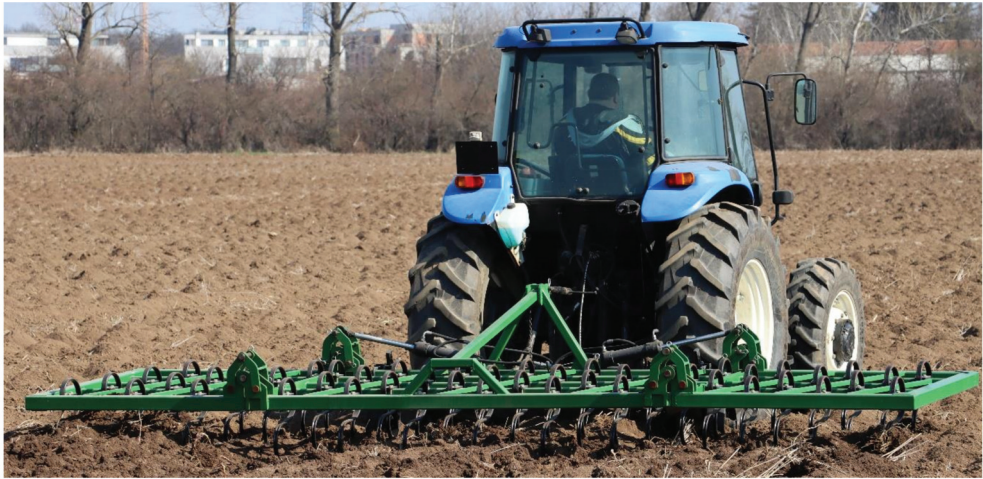
Figure 1. The MCLS complex cultivator operates in the version with a working width of 4 m.
