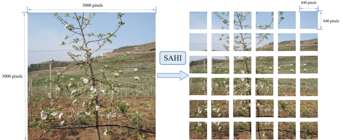
Figure 3. The process of SAHI splitting the original image.
