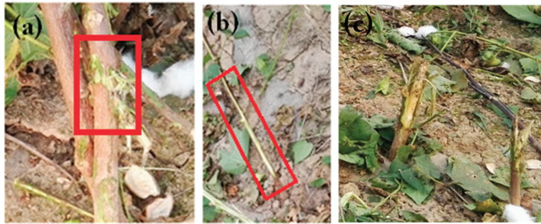
Figure 12. Conditions of the cotton stalk epidermis following a stalk extraction attempt. (a) Example of the epidermis following successful cotton stalk extraction. (b) Example of the epidermis of a cotton stalk that failed to be extracted. (c) Example of the epidermis of broken cotton stalks.
