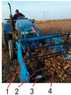
Figure 13. Field test photo: 1. Reel wheel 2. V-shaped tooth roller 3. Torque transducer 4. Cotton stalks.
