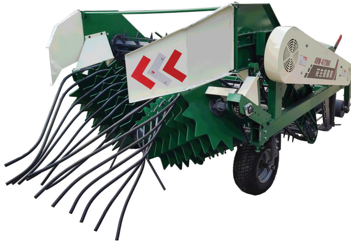
Figure 3. Peanut digger-inverter experimental machine.
