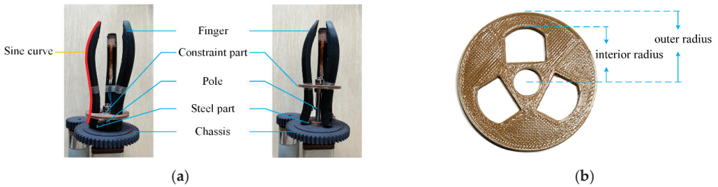
Figure 2. The design of gripper: (a) opening and closing of gripper; (b) the constraint part.
