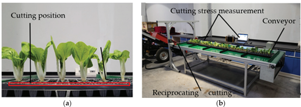
Figure 5. Schematic diagram of measurement system of cutting stress: (a) test sample; (b) cutting stress measurement system.
