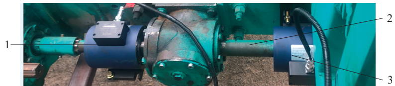
Figure 1. Physical view of header power sensor. 1: power sensor of inside shaft 2: T-type drive shaft 3: power sensor of outside shaft.
