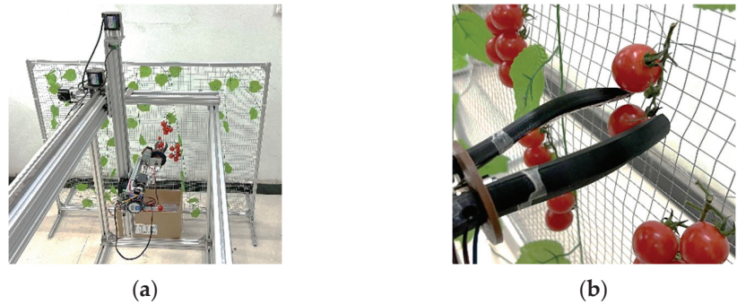
Figure 15. Experiment of cherry tomatoes picking: (a) The system of picking robot; (b) Gripper picking.
