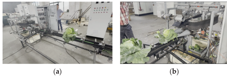
Figure 18. Operation performance test: (a) conveying system of cabbage; (b) harvesting system of cabbage.
