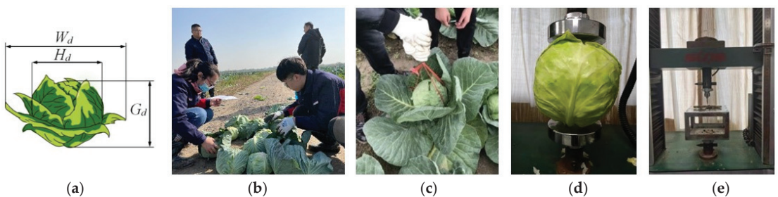
Figure 1. Determination of basic physical parameters and harvesting mechanical properties test of cabbage: (a) Physical characteristics acquisition: 1: W_d : Expansion degree 2: H_d : transverse diameter 3: G_d : vertical diameter (b) Physical characteristics acquisition process. (c) Determination of pull-out force. (d) Compression test. (e) Root cutting force test.
