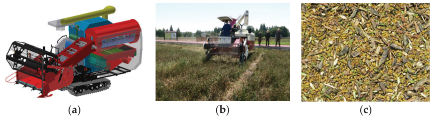
Figure 9. Combined Chinese milk vetch seed harvester and field test process. (a) Three-dimensional diagram of the combined Chinese milk vetch seed harvester. (b) Chinese milk vetch field harvest test. (c) Materials in the seed bin.
