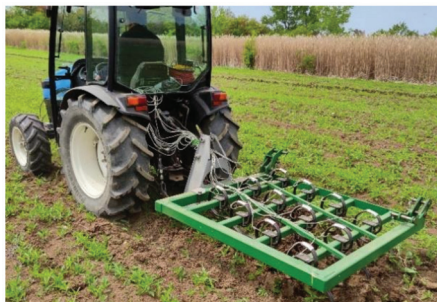
Figure 3. MCLS in operation in the 1 m working width variant.
