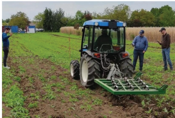
Figure 6. MCLS variant with a working width of 1 m in operation with a 45 HP tractor.
