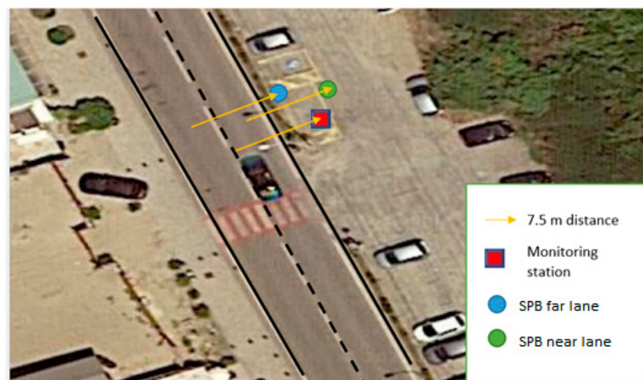
Figure 2. Measurement setup in T1 (Marina di Pisa). Near lane is the one close to the traffic counter and monitoring station; far lane is the one in the opposite direction.
