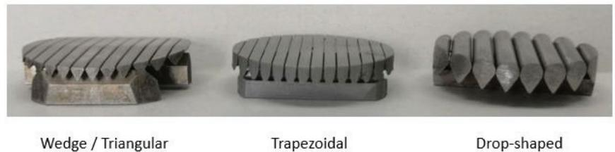
**Figure 3.** Wire-wrapped screens with different wire profiles [by authors] (wires are welded to elements of longitudinal supporting ribs).
