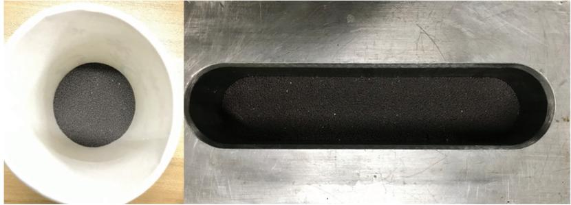
**Figure 4.** Pure proppant and its placement in the diversion chamber.
