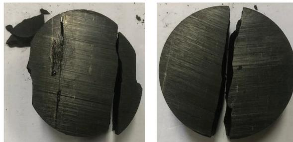
**Figure 7.** Fragmentation morphology of loaded shale in different bedding directions.
