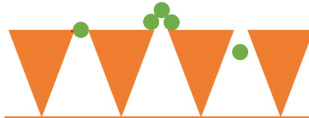
**Figure 10.** Wedge/Triangular wire profile and its interaction with particles.
