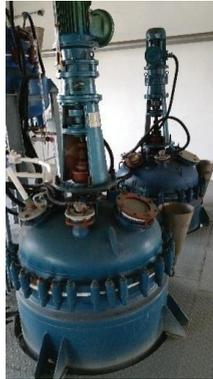
**Figure 1.** Plugging agent synthesis reactor.
