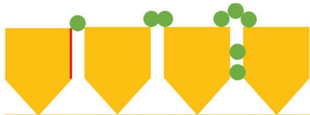
**Figure 11.** Trapezoidal wire profile and its interaction with particles.
