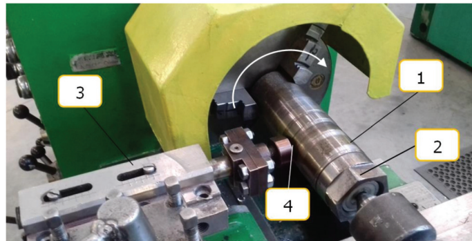
Figure 1. View of the test stand used in the experiment: 1: specimen; 2: mandrel with mounted samples; 3: slide burnishing tool; 4: diamond tip with radius R .
