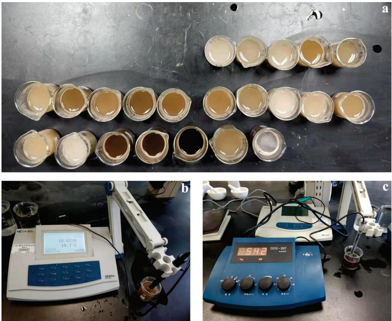
Figure 3. Measurements of main chemical soil properties. (a) Prepared soil suspensions; (b) pH measurement process; (c) EC measurement process.
