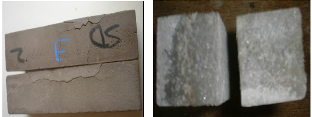
Figure 12. Beam of dune sand mortars immersed in sodium sulfate solution (5%) at 180 days [73].
