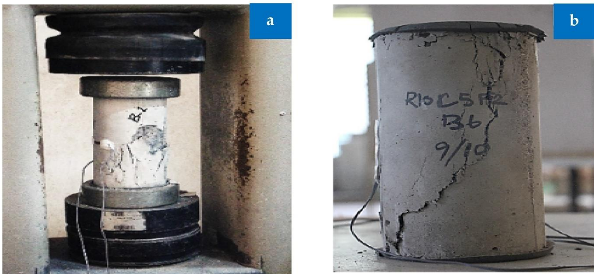
Figure 14. Cylinder failure under compression: (a) reference and (b) combination of RCA, rubber, and fibers [44]: used as per Elsevier permissions.
