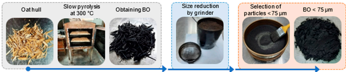
Figure 2. BO production sequence.
