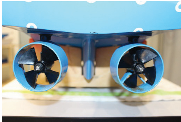
Figure 2. Tito Neri azimuthing thrusters from stern.
