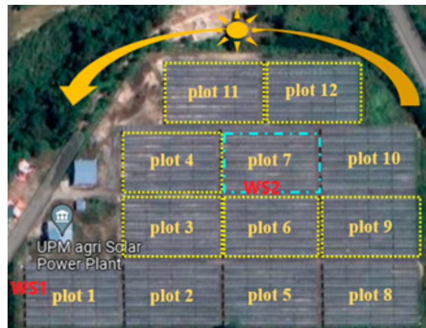
Figure 5. Google map layout of LSS PV farm in Puchong, Selangor (five acres). WS is the location for Weather Station.
