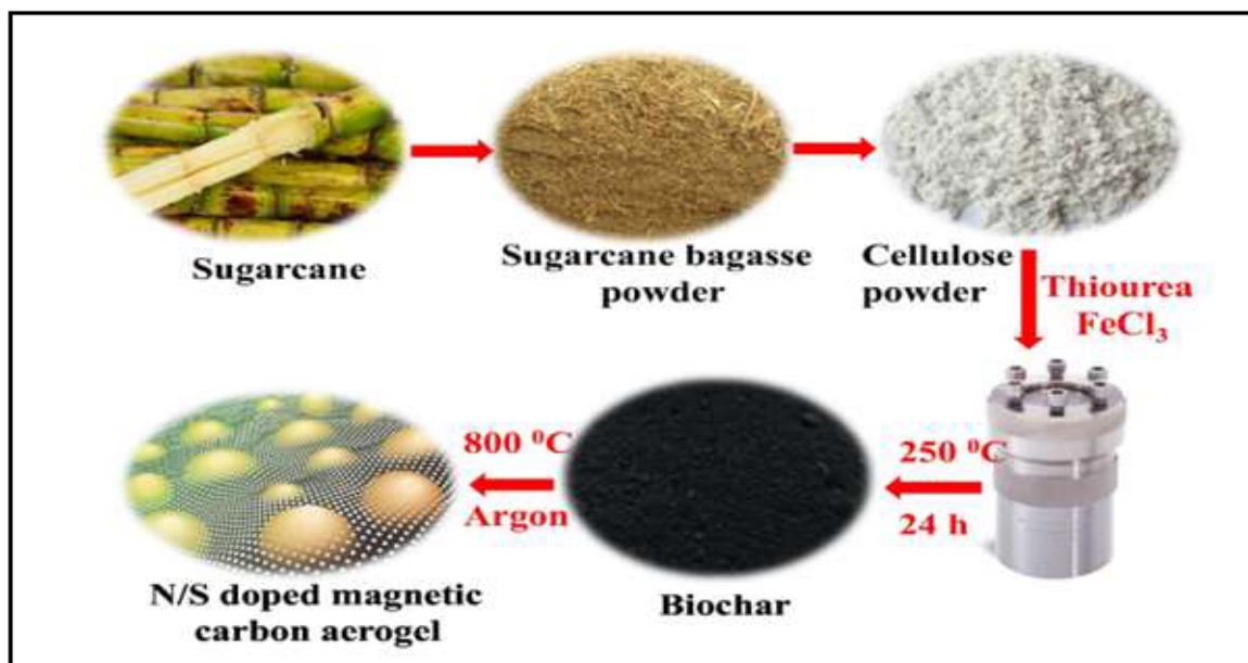
Figure 9. The fabrication of N/S doped carbon aerogel by using sugarcane bagasse for bisphenol-A adsorption. Adapted from Ahamad et al. [125].
