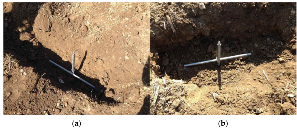
Figure 16. Continuous pipe foundation for field test. (a) Steel wire, (b) steel plate [23].
