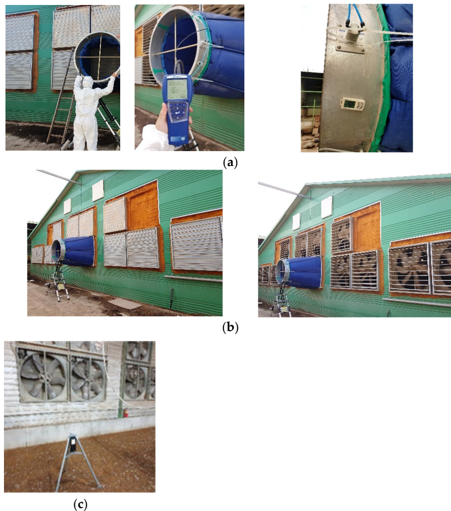
Figure 6. Measurement the ventilation flow rate of the broiler house of exhaust fan: (a) Installation of an air flow meter in the tunnel exhaust fan; (b) Ventilation flow rate change according to the number of fans; (c) Internal static pressure of exhaust fan.
