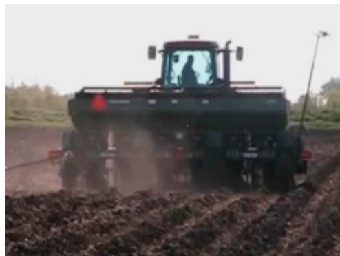
Figure 17. Lockwood 506 series potato planter. Reprinted with permission from ref. [48] Copyright 2018 Lockwood Industries.
