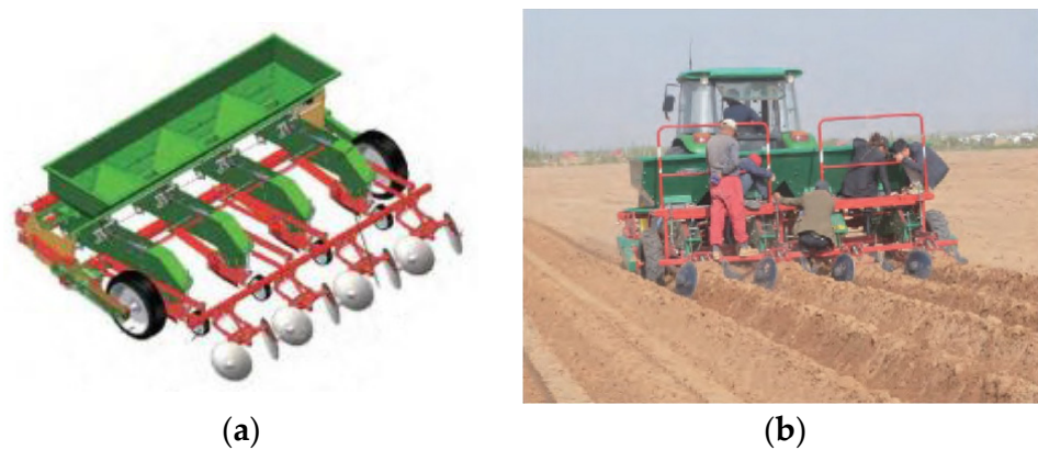
Figure 14. Vibration-arranging-based planter. (a) The structure of vibration-arranging-based planter. Reprinted with permission from ref. [63]. Copyright 2019 China Agricultural University. (b) The working process of the vibration-arranging-based planter. Reprinted with permission from ref. [63]. Copyright 2019 China Agricultural University.
