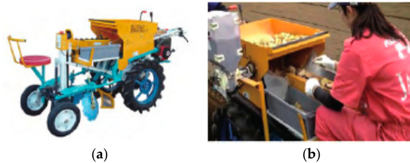
Figure 19. JAGIRL man-aided potato planter (a) The structure of planter. Reprinted with permission from ref. [13] Copyright 2019 JAGIRL Industries (b) Manual assisted operation. Reprinted with permission from ref. [13] Copyright 2019 JAGIRL Industries.
