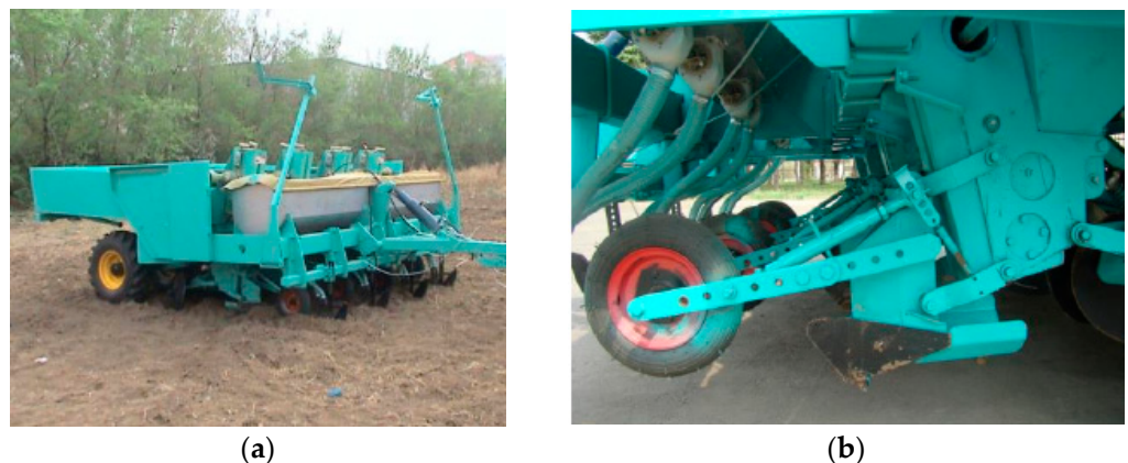
Figure 28. Two views of the 2CMW-4B planter and the depth control device. (a) Operation process of the device; (b) Structure of ditching and seeding device. Reprinted with permission from ref. [99]. Copyright 2019 Shandong University of Technology.
