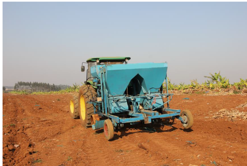
Figure 4. HN 2CZD-2 single-bud sugarcane planter.
