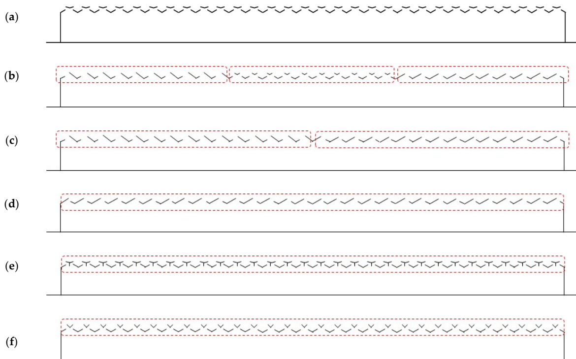
Figure 6. Schematic depicting the improved model ventilation structure of the CR-venlo greenhouse with continuous roof vents: (a) Case 0: CR-venlo greenhouse, (b) Case 1: Opening of windward roof vents at 1–5 span and leeward roof vents at 11–15 span, (c) Case 2: Opening of windward roof vents at 1–7.5 span and leeward roof vents at 7.5–15 span, (d) Case 4: Opening of all windward roof vents, (e) Case 4: Windbreak installation in the center of all roof vents, (f) Case 5: Increasing the opening angle of roof vents.
