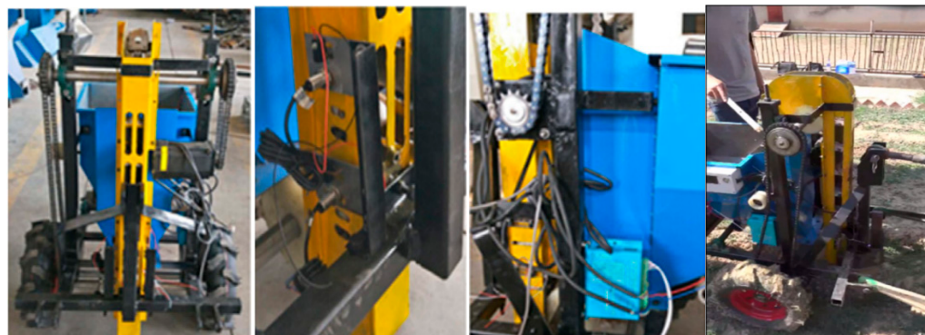
Figure 23. Integrated seeding and compensating potato planter based on one-way clutch. Reprinted with permission from ref. [96]. Copyright 2019 Gansu Agricultural University.
