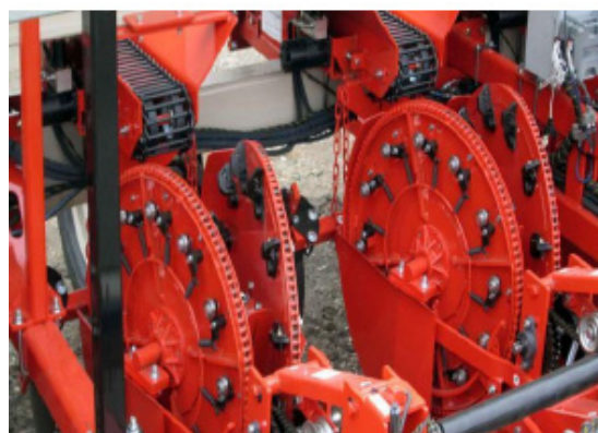
Figure 15. Lockwood 6200 Needle-type potato planter. Reprinted with permission from ref. [48] Copyright 2018 Lockwood Industries.
