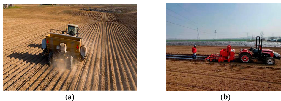
Figure 32. Automatic Potato planter with GPS system. (a) Double L planter works under GPS navigation. Reprinted with permission from ref. [12]. Copyright 2021 Double L Industries. (b) Navigation test of planter.
