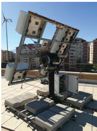
Figure 8. The designed high-concentration photovoltaic system (HCPV) tracker.
