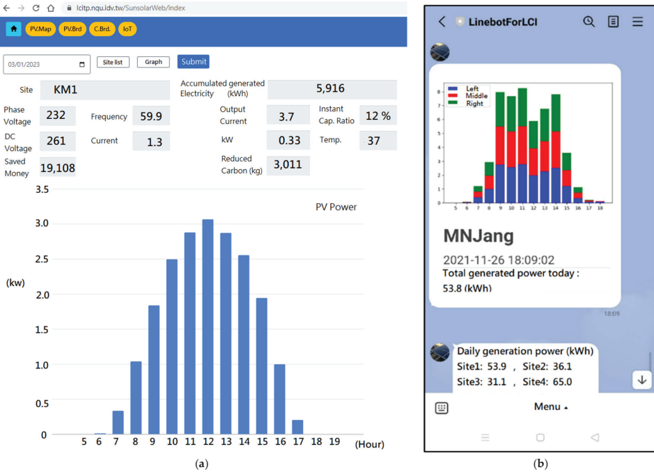
Figure 13. (a) Desktop web GUI, (b) smartphone line bot GUI. Both show PV daily data.
