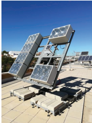
Figure 7. The designed high-concentration photovoltaic system (HCPV) tracker.
