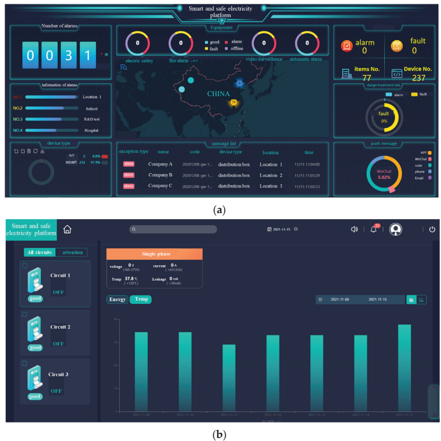
Figure 9. Circuit breaker digital monitoring system. (a) The main interface. (b) Circuit breaker monitoring interface.
