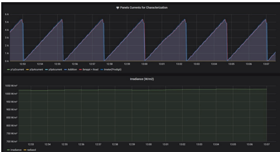
Figure 12. Detailed view of Grafana GUI to observe PV current and irradiance during characterization.
