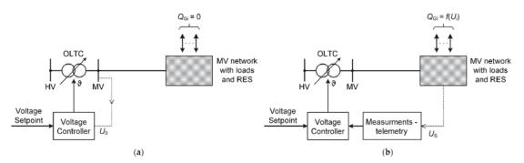
**Figure 4.** Simplified methods of voltage control in the MV grid with distributed generation: (**a**) traditional regulation—keeping a constant voltage value on the MV busbars, (**b**) keeping a constant voltage value in an optimally selected node deep inside the grid and activating the characteristics of Q(U) inverters.
