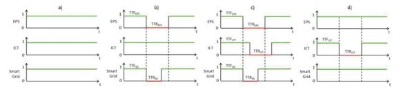
**Figure 5.** Methodology of smart grid co-simulation: (a) EPS, ICT and Smart Grid in operation, (b) outage in EPS, ICT in operation, shortening the failure in Smart Grid, (c) failure in EPS, failure in ICT, shortening the failure in Smart Grid, (d) EPS in operation, failure in ICT, Smart Grid in operation [80,81].
