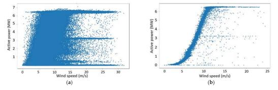
Figure 10. Wind power curves. (a) Original 1s data (b) and 10 min resampled data.
