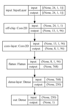
Figure 2. SNN model architecture.
