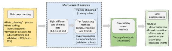
Figure 8. A general diagram of the consecutive steps in the forecasting process.
