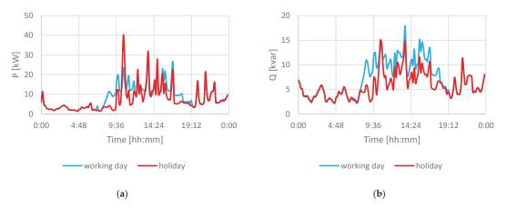
Figure 5. (a) Total daily active power demand characteristics of the test microgrid; (b) Total daily reactive power demand characteristics of the test microgrid.
