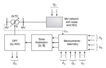
**Figure 1.** Diagram of the OPFh-MVt voltage control method, control signals—transformer ratio  $\vartheta$  and reactive power of RES systems.
