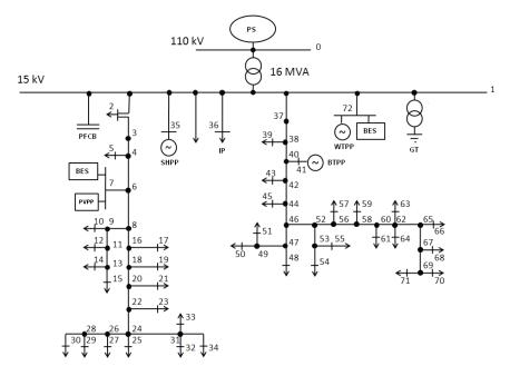
Figure A3. Rural MV distribution network with the distributed generation sources (PS—power system, PVPP—photovoltaic power plant, BES—battery energy storage, SHPP—small hydropower plant, BTPP—biogas-turbine power plant, WTPP—wind-turbine power plant, PFCB—PFC capacitor bank, GT—grounding transformer, IP—industrial park).
