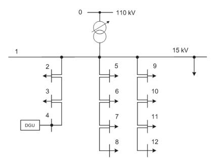
Figure A5. Actively managed MV distribution network with the DG unit (based on [84]).
