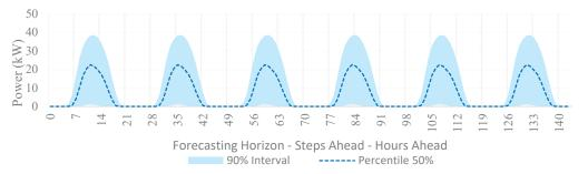
**Figure 4.** The dashed dark blue line represents the mean, and the light blue area represents the 90% interval probability distribution of power for the CH-PeEn benchmark for the target PV system for six consecutive days.
