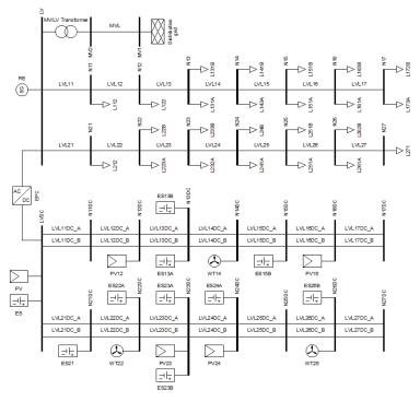
Figure 4. Schematic diagram of the test microgrid.
