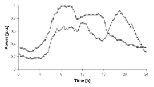
**Figure A2.** Typical daily load profile (15-min intervals) for residential consumers (a line with the triangles) as well as industrial parks and electric traction substation (a line with the quadrants); based on [85].
