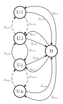
**Figure 2.** N + 1-state reliability model of a renewable generation system. *U.i* is an up unit state (normal operation) with *i*-th of *n* level of energy carrier  $\{1, ..., i, j, ..., n\}$  and *D* is a down unit state (failure).
