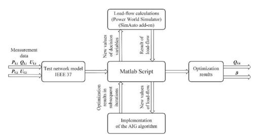
Figure 3. General scheme of the organisation of the computational process used in solving the optimisation task.
