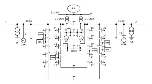
**Figure A1.** MV urban distribution network with the distributed generation sources (PS—power system, PVPP—photovoltaic power plant, BES—battery energy storage, MT—micro-turbine, GTPP—gas-turbine power plant, GT—grounding transformer, MVUS—MV urban distribution substation, IP—industrial park).
