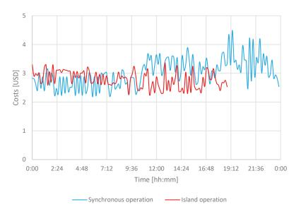
Figure 8. Daily changes of costs of operation of the hybrid test microgrid.
