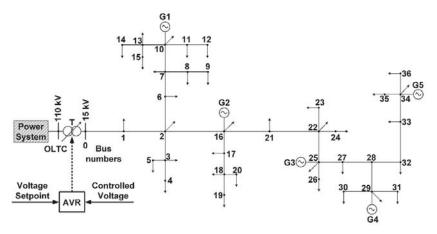
Figure 6. IEEE 37 test network diagram [86].
