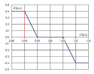
**Figure 5.** The Q(U) characteristic of the inverter of the RES installation (photovoltaic and wind farm) selected for the analysis of the effectiveness of the voltage regulation in the MV grid.
