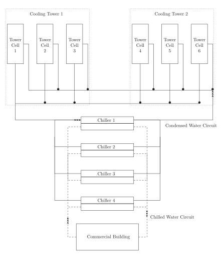
Figure 1. Refrigeration system's configuration.
