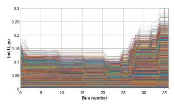
**Figure 15.** The results of the simulation assessment of the voltage quality indicator Ind U for the IEEE 37 network depending on the selection of the reference node, the voltage of which is maintained at a given level by the OLTC controller.
