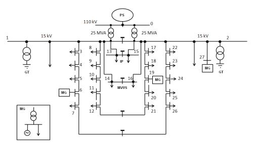
Figure A4. MV distribution network with connected LV microgrids (PS—power system, MG—microgrid, IP—industrial park, MVUS—MV urban distribution substation, GT—grounding transformer).
