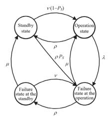
**Figure 1.** Four-state reliability model of a conventional generation unit operating in peak service.  $P_S$  is a probability value of unsuccessful unit starting,  $\nu$  is an operation rate,  $\rho$  is a standby rate,  $\lambda$  is a failure rate and  $\mu$  is a repair rate [63].
