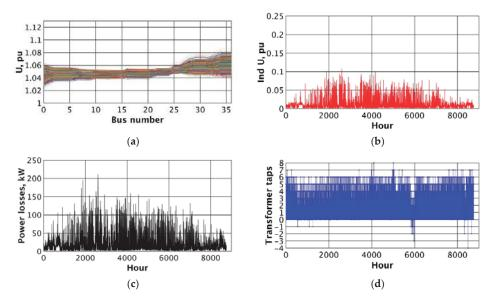
**Figure 10.** Results of the analysis of the effects of voltage regulation using the OPFh-MVt method: (a) voltage values in the network nodes for all hours of the year, (b) annual changes in the voltage quality index, (c) annual changes in power losses in the network, (d) annual changes in the position OLTC.
