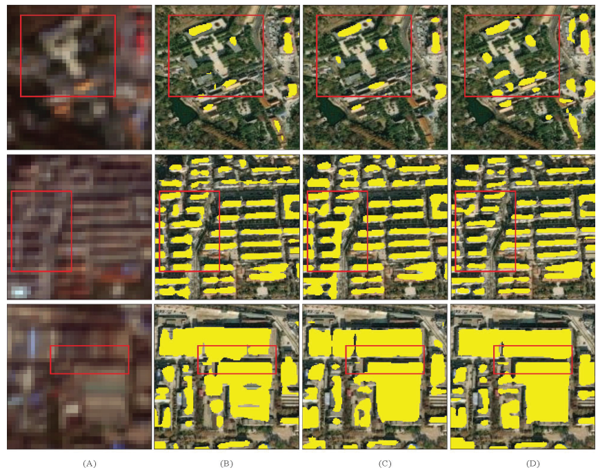
Figure 13. Examples of the super resolution and then semantic segmentation results obtained by the different methods in Sentinel-2 images. (A) The image tile (10 m/pixel). (B–D) The building extraction results (2.5 m/pixel) from ESPC_NASUnet, FSRSS-Net, and our SGFANet under the SR-then-SS framework, respectively. For better visual effects, we used the 2.5 m image from Esri community as the base map. The red squares indicate our notable improvement.
