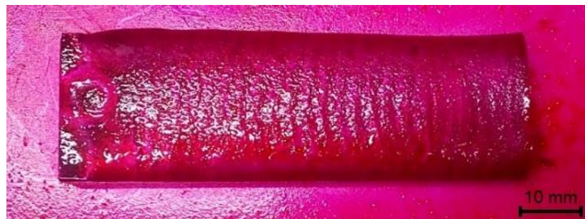
Figure 4. View of the sample during the penetrant testing (PT).
