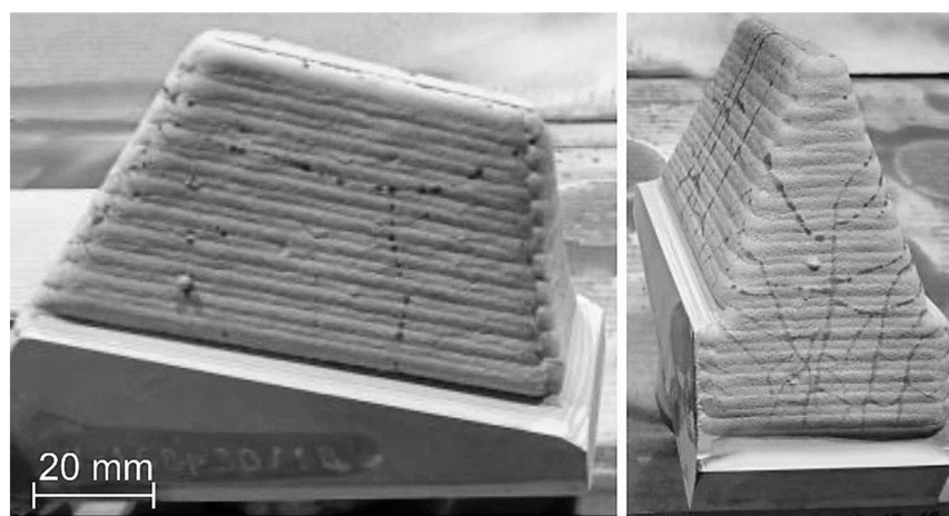
Figure 21. View of the tooth surface of the prototype three-bite auger filled with LDMD with a designed composite filler.
