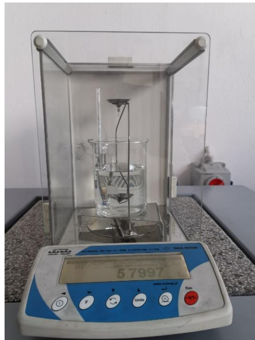
Figure 5. View of an analytical balance for density of the deposited layer measurement.
