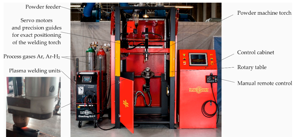
Figure 3. Gap automated unit robotic coating system.
