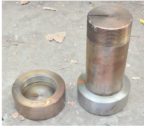
Figure 3. Cook-off bomb after tests.
