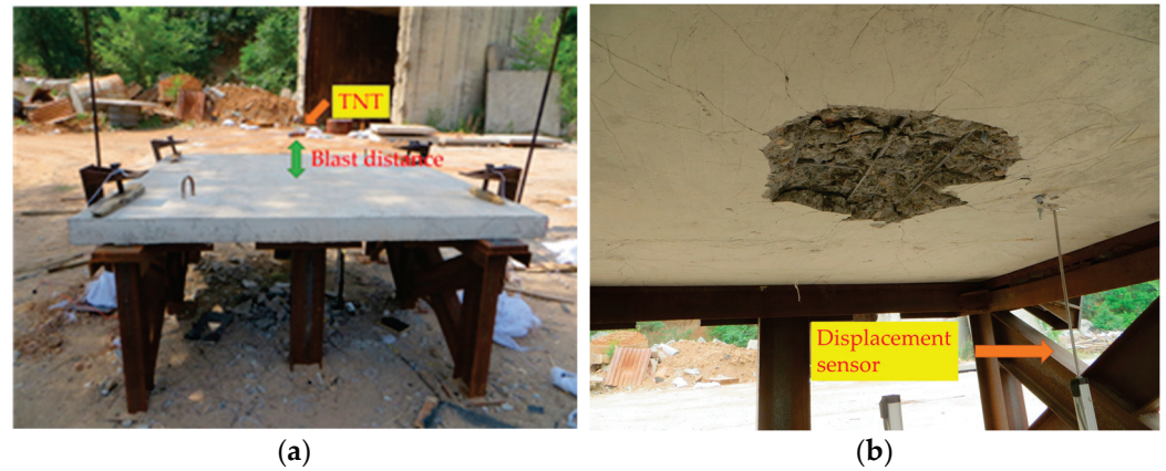
Figure 2. Experimental layout diagram. (a) Overall layout of the experiment; (b) arrangement of displacement sensor.
