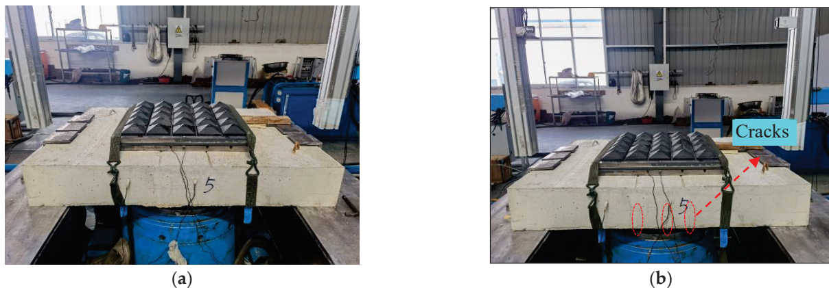
Figure 5. Damage condition of the specimen after a single impact. (a) Before the test; and (b) After the test.
