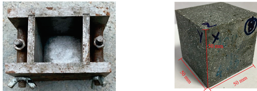
Figure 1. Trial mold and test specimen.
