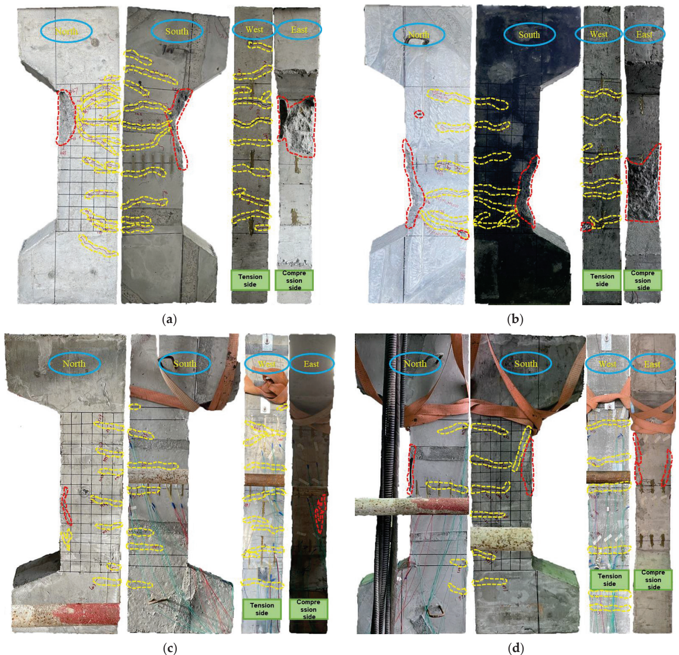
Figure 8. Typical failure modes of RC columns: (a) FITRC45-2 column specimen; (b) CRC45 column specimen; (c) FITRC35-2 column specimen; (d) CRC35 column specimen.
