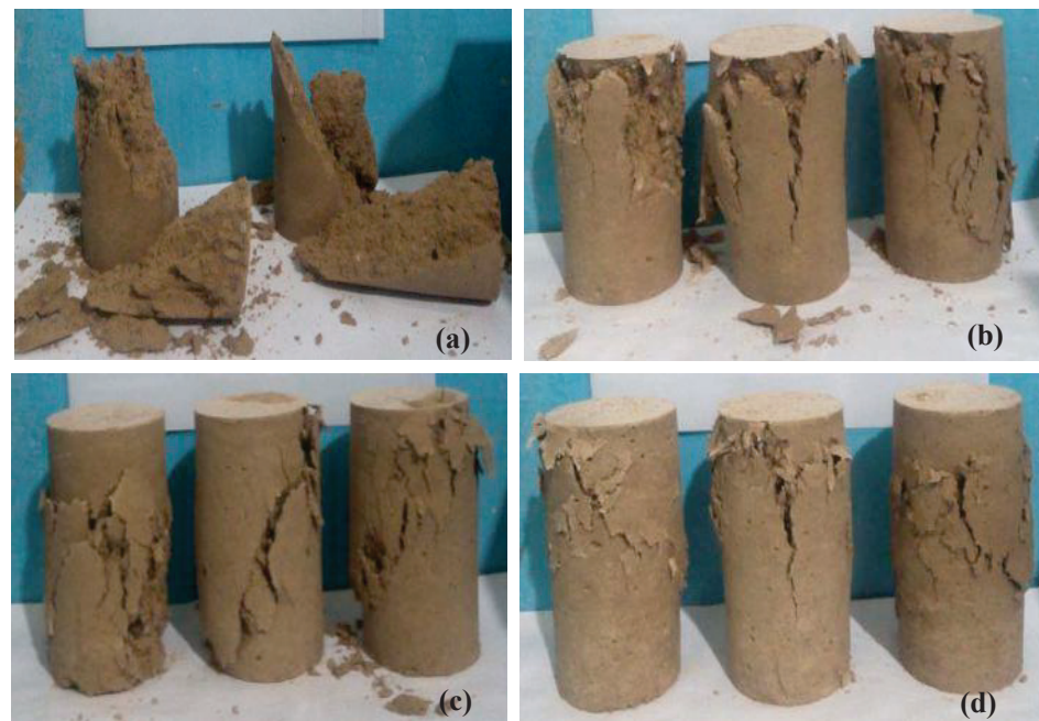
Figure 3. A view of 28-day, ambient-cured specimens after failure: (a) 0%, (b) 0.5%, (c) 1%, and (d) 2% fiber content.
