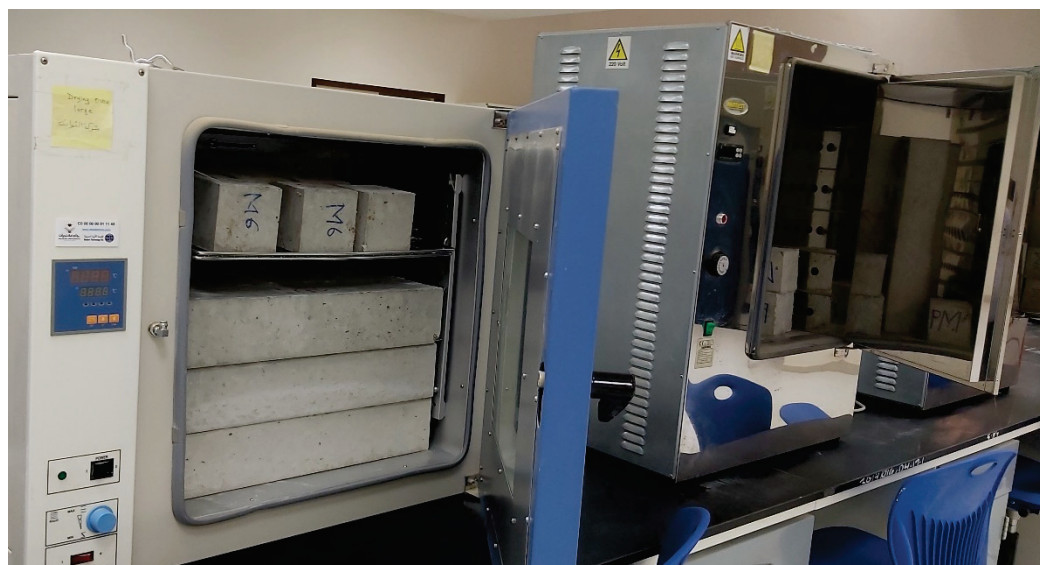
Figure 4. Fiber reinforced concrete specimens under heat–cool cycles.
