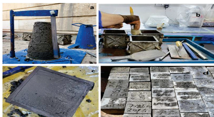
Figure 1. (a) Slump test, (b) mold preparation, (c) a typical casted specimen, (d) cured specimens.
