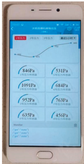
Figure 10. Internet of things measurement system—mobile terminal.
