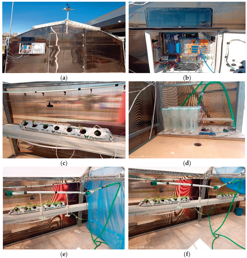
Figure 10. (a) Exterior view of the application greenhouse. (b) Internal view of the control board. (c) View of the strawberry plants, including irrigation system, webcam, and spraying sprinklers. (d) Four different spraying tanks, mixing tank, and control system. (e) General view of the application system with the humidification system included. (f) System controlled by deep learning and normal system view.
