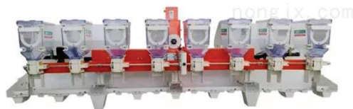
Figure 1. Datong 2BD-8A (DXD830) rice direct seeding machine.
