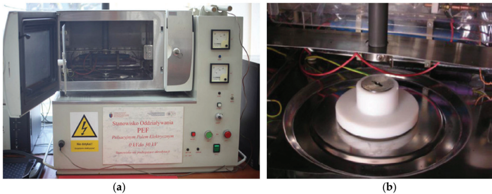
Figure 1. Ertec Su-1 test stand: (a) discharge chamber; (b) stationary sterilization cell.
