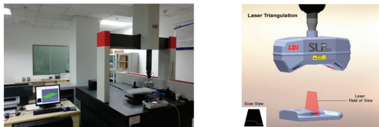
Figure 7. LDI-Surveyor ZS/SLP ultra-high accuracy high-speed 3-D laser scanning system and the structure of scanning probe.
