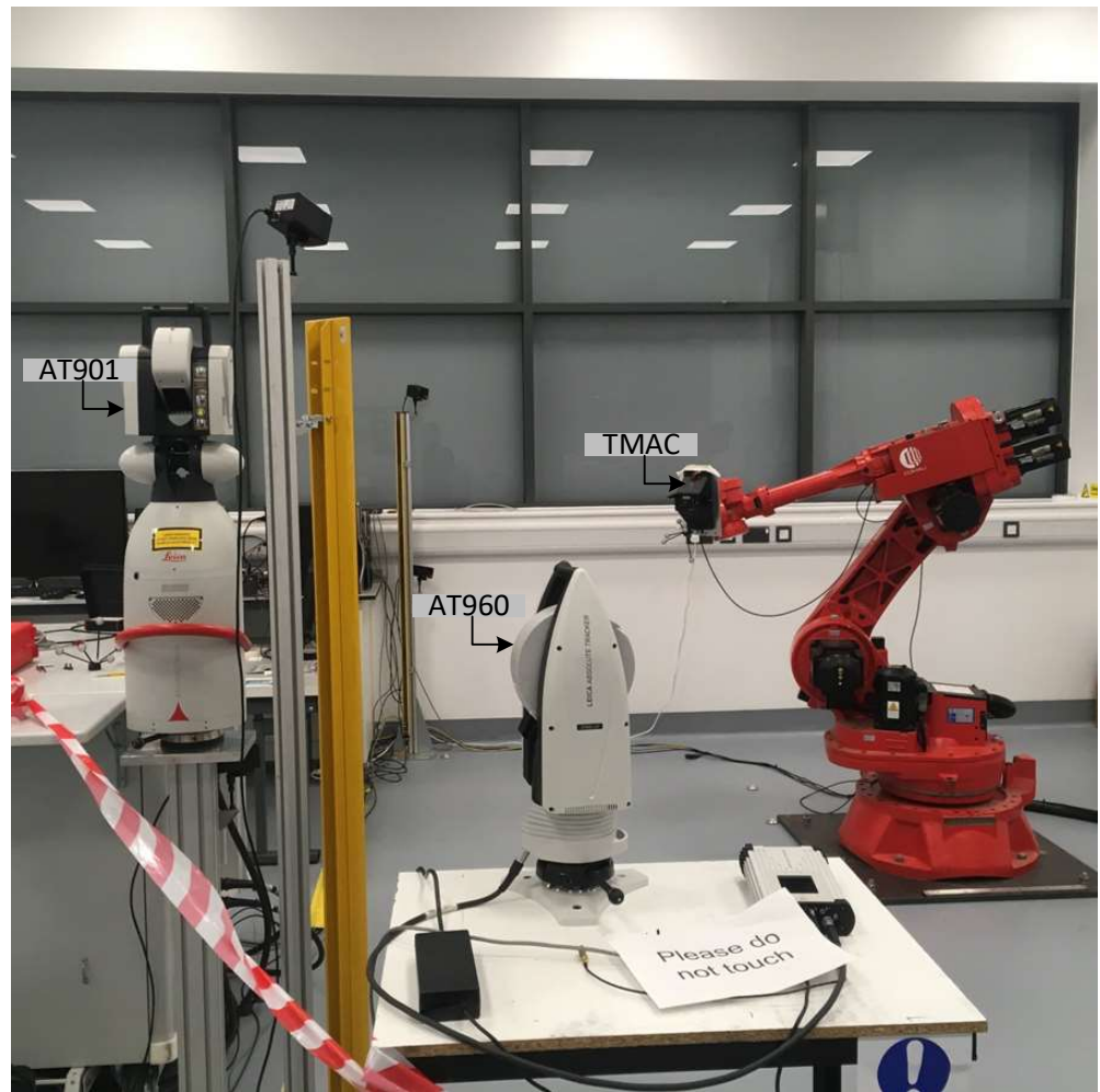
Figure 16. AT960 Leica Tracker Setup for NRTEC Verification.
