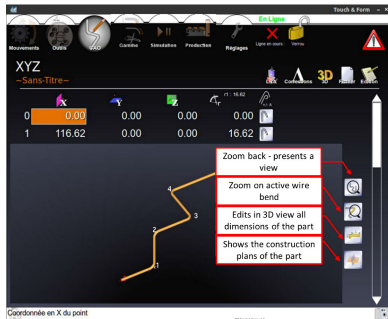
Figure 3. 3D view of the wire in the equipment console.
