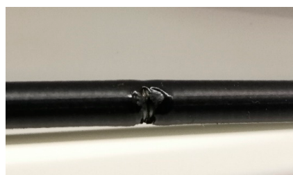
Figure 7. Laser cutting test results for the laminated spiral without inner tube.
