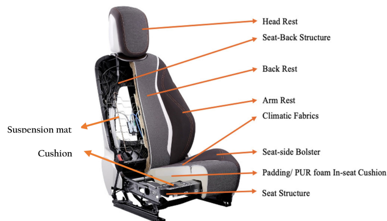
Figure 1. Components of a car seat (adapted from [38]).
