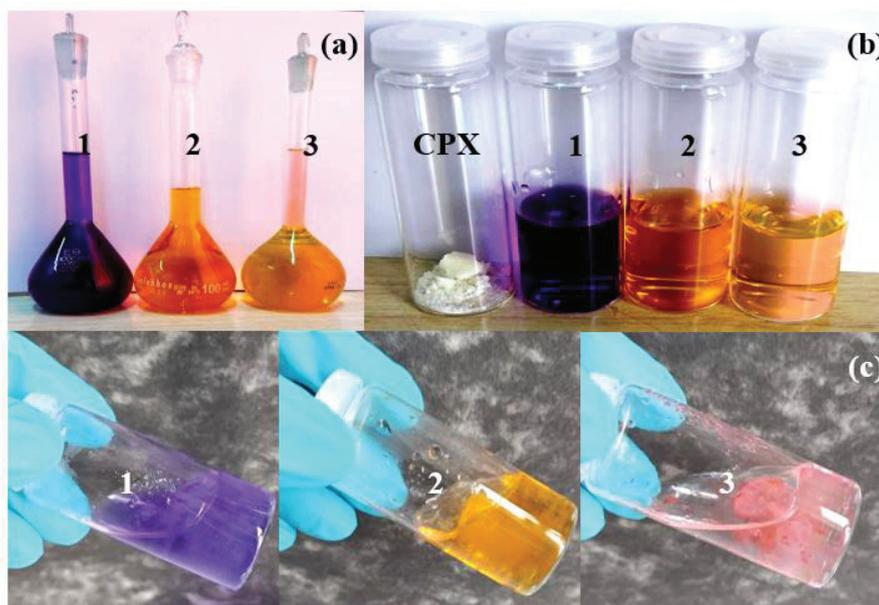
**Figure 10.** Visual dye preliminary adsorption tests of CPX hydrogel. (1) Gentian violet; (2) methyl orange; and (3) eosin; (a) stock solution; (b) initial time; (c) after 24 h.
