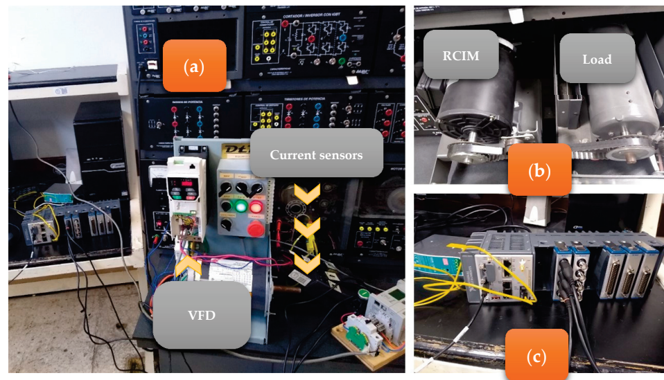
Figure 5. Laboratory test system. (a) Full system. (b) RCIM under analysis and its load. (c) National Instruments data acquisition system compact RIO.
