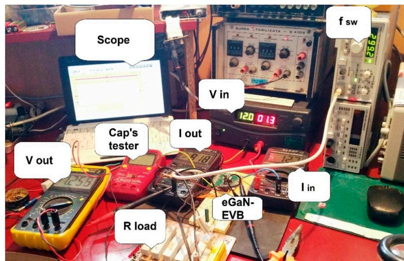
Figure 11. General view of the experimental set-up. Voltage waveforms were displayed using an USB-DSO oscilloscope—ISDS 220B and a CP-05+ current probe.
