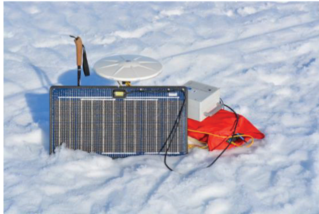
Figure 3. Static GNSS measurement during GKE 2015.
