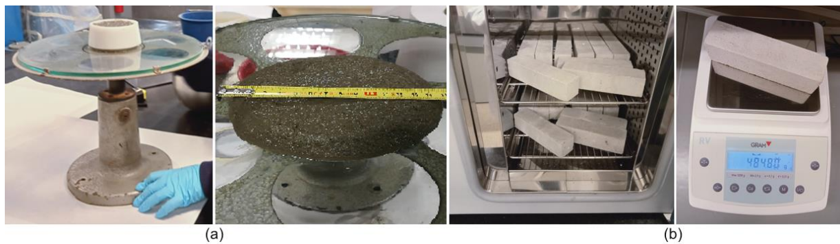
Figure 3. (a) Workability measurement, (b) testing of the dry bulk density of hardened mortars.
